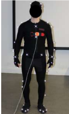
(a) Human subject with IMU attached to the torso
