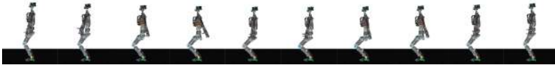
(b) The simulated ARMAR-4 performing a squatting motion under LQR whole-body control
