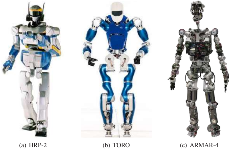
Figure 2.3: (a) The velocity-controlled HRP-2 (taken from [Kaneko et al. 2004], © 2004 IEEE), (b) the torque-controlled TORO (adapted from [Engelsberger et al. 2014b], © 2014 IEEE) and (c) the torque-controlled ARMAR-4 humanoid robot.
