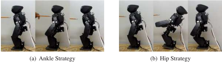
Figure 3.2: A DARwin-OP humanoid robot reacting to a push from the front by (a) actuating its ankle joints (ankle strategy) and (b) bending its hip (hip strategy). Adapted from [Hyon et al. 2009], © 2009 IEEE.
