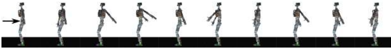
(a) The simulated ARMAR-4 reacting to a frontal push under LQR whole-body control
