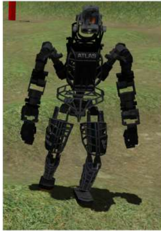
Figure 3.3: A simulated Atlas robot walking over uneven terrain under torque-based QP control, following a previously generated trajectory (taken from [Feng et al. 2013], © 2013 IEEE).
