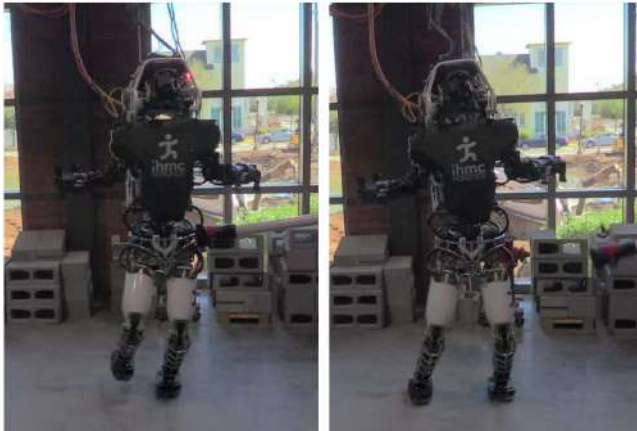
Figure 3.10: An Atlas humanoid robot reacting to a lateral push by quickly stepping to the side (taken from [Griffin et al. 2017], © 2017 IEEE).
