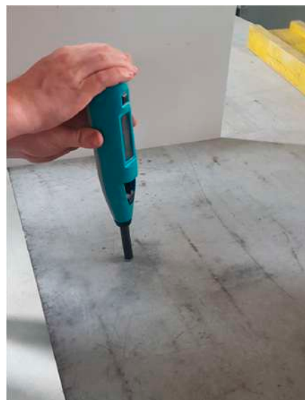
Figure 6. Schmidt hammer when testing the repeatability on a 30 cm thick concrete slab (used as reference material).
