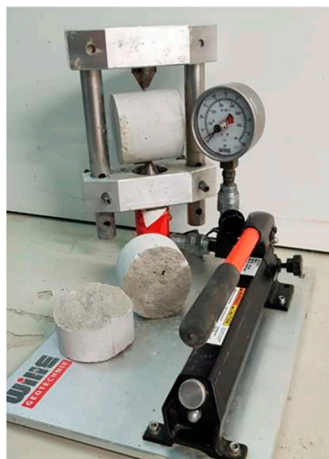
Figure 7. Point load testing on concrete mortar cylinders (used as reference material).
