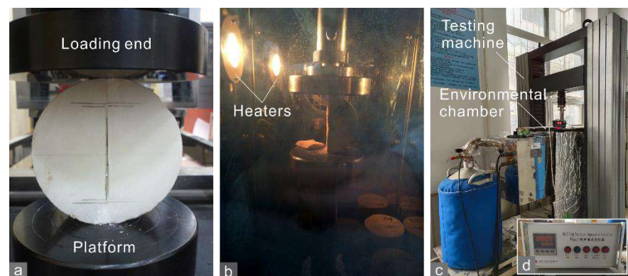
Figure 3. (a) CCNBD test on a marble A specimen at room temperature; (b) BD test on a sandstone specimen in the chamber at 125 °C; (c) MTS servo-control testing machine, SNAS GDS-300 environmental chamber, and (d) WK650 temperature controller.
