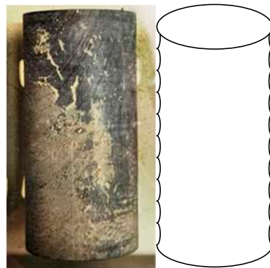
Figure 5. Photograph and schematic diagram of surface damage after chemical solvent erosion.
