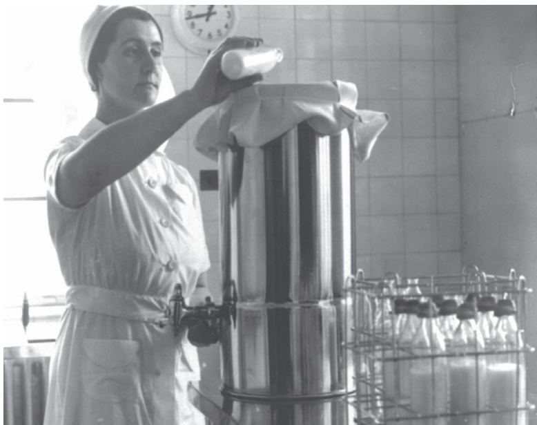
Figure 2.2 We are told that the milk is filtered through eight layers of gauze into a chromium-plated cylinder. Source: Reprinted with permission from Historic England.
