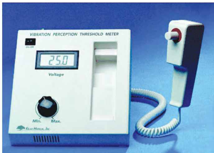
FIGURE 26.3: Vibratory Perception Threshold Monitor (VBT)
