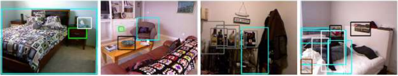
Figure 2.11: Detection of affordances in RGB images using an end-to-end CNN (taken from Ye et al. 2017, © 2017 IEEE).
