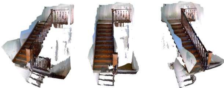
Figure 3.4: Cropped visualization of a registered point cloud resembling a handrail-equipped staircase. The point cloud has been registered using RTAB-Map (Labbé et al. 2014) from a set of 64 individual point clouds.
