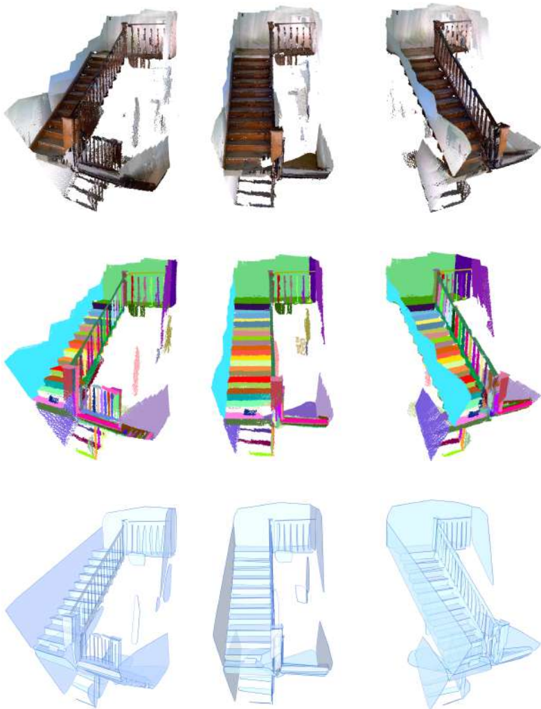
Figure 3.5: Geometric primitives extracted from a manually segmented, registered point cloud of a staircase. The visualizations show the original point cloud ( first row ), the manually created segmentation ( second row ) and the resulting set of planar geometric primitives ( third row ).
