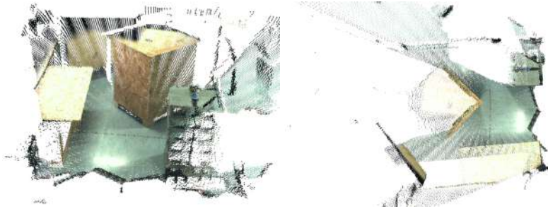
Figure 3.3: A single exemplary LIDAR point cloud captured in a test environment for locomanipulation for the humanoid robot WALK-MAN. Although the laser scan produces an extensive depth image of the environment ( left ), shadowed areas are not reflected in the point cloud ( right ). For obtaining a complete point cloud representation of the environment, multiple views from different positions need to be captured and registered.
