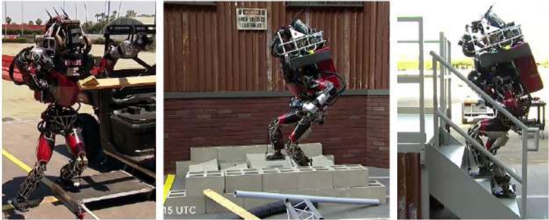
Figure 2.14: The humanoid robot Atlas of the team WPI-CMU performing different tasks of the DRC Finals, i. e. utility vehicle egress, walking over rough terrain and staircase climbing (taken from Atkeson et al. 2015, © 2015 IEEE).
