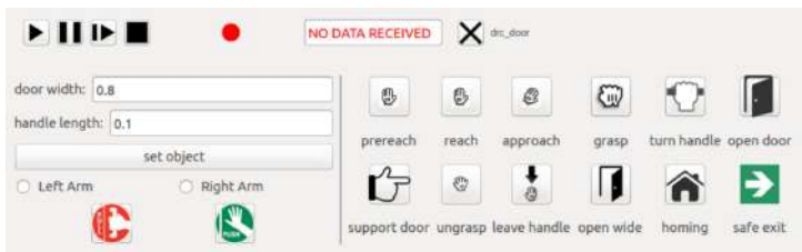
Figure 2.15: Parts of the task-specific pilot interface of the team WALK-MAN for the door-opening task (taken from Tsagarakis et al. 2017, © 2017 Wiley Periodicals, Inc.).
