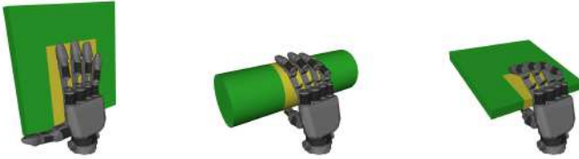
Figure 5.1: Visualization of grasp volumes (yellow) for exemplary grasps on planar and cylindrical primitives (green).
