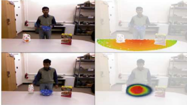
Figure 2.9: Visualization of affordance heatmaps for placeability (top) and purability (bottom) (taken from Koppula et al. 2016, © 2016 IEEE).
