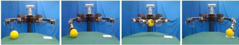
Figure 2.7: Developmental learning of manipulation affordances and associated control policies in a tabletop scenario (taken from Hart et al. 2011, © 2011 IEEE).
