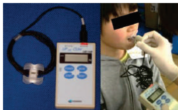
Figure 9. Lip closure force measurement. The lip closure force was measured using a Lip de Cum ® LDC-110R (Cosmo Instruments Co. Ltd., Tokyo, Japan). The subjects were seated with the Frankfurt horizontal plane parallel to the floor. Duckling lip holders were placed between the lips and the maximum lip closure force was measured in the intercuspal position.
