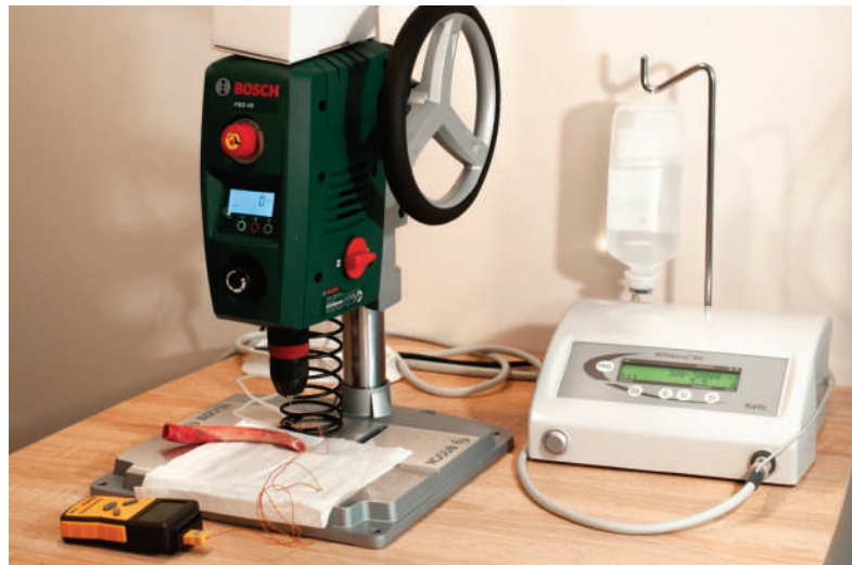
Figure 4. The study setting, including the bench drill, and the irrigation system (provided by the surgical unit).
