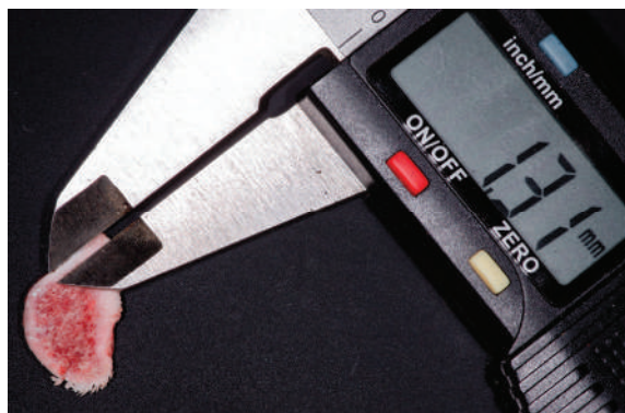
Figure 1. Porcine rib model used for the in vitro experiment with a cortical bone thickness of 1.31 mm.
