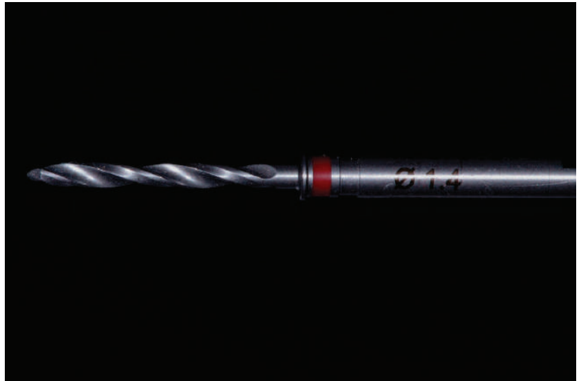
Figure 2. 1.4 mm diameter drill used for the investigation.
