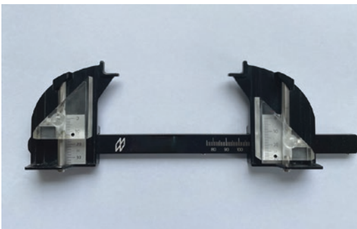
Fig. 7.2 Parallax-free exophthalmometer according to Mourits
