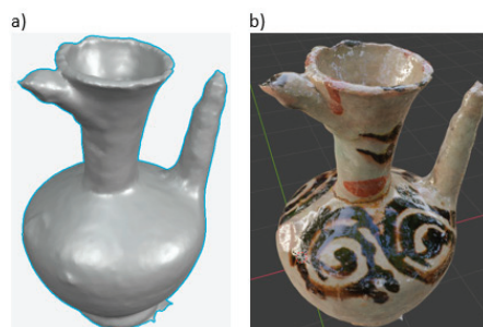
Figure 12. The appearance of the digital 3D model of the jug obtained by the SfM method after smoothing the surface: (a) without texture, (b) with texture.
