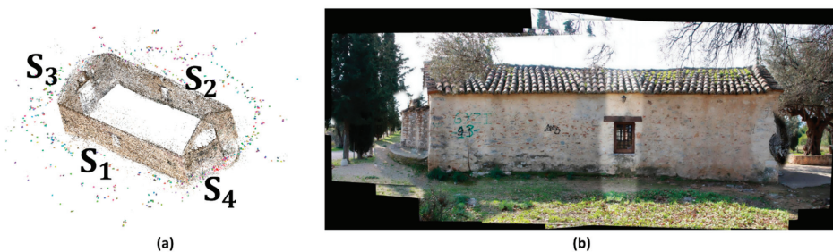
Figure 9. Steps in the orthophoto generation process for the Church of Agios Nikolaos: (a) the point cloud generated and its four major façade planes; and (b) a representative orthophoto generated from S_1 .
