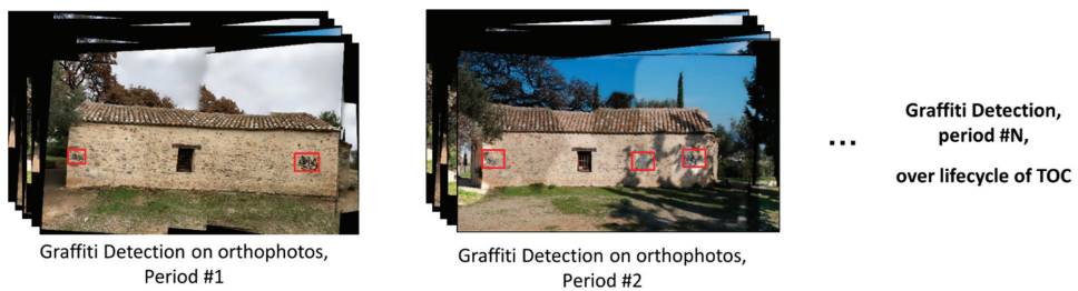
Figure 5. The robust graffiti detector was applied to each of the orthophotos, providing an overall presence of graffiti, including the location and size of each mark.
