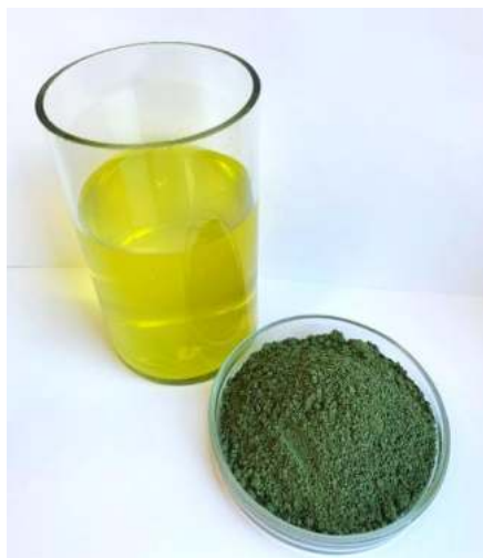
Figure 1. Liquid and solid phases of catalyst slurry.
