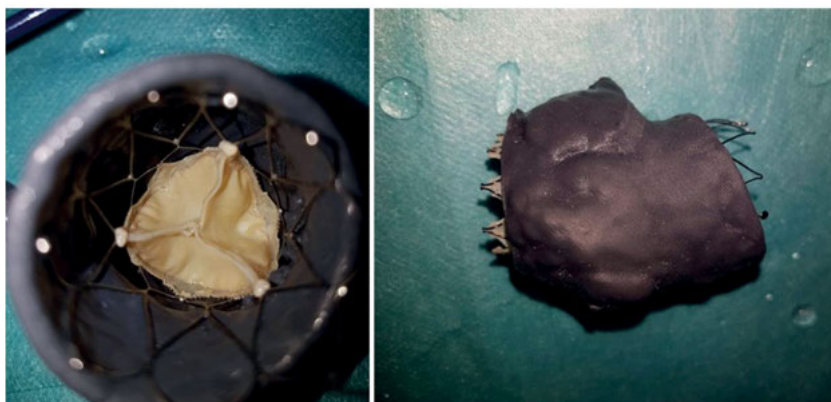
Fig. 5.2: Model of aortic root 3D printed with stereolithography technique. Semiflexible resin allowed the simulation of transcatheter aortic valve implantation (TAVI) and proper valve sizing. Model was created in 2017 for cardiologists from Warsaw Medical University (Warsaw, Poland).
