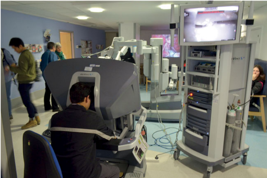
Fig. 9.5: Surgeon console in the da Vinci robot system https://upload.wikimedia.org/wikipedia/commons/6/68/Cmglee_Cambridge_Science_Festival_2015_da_Vinci_console.jpg . This file is licensed under the Creative Commons Attribution-Share Alike 3.0 Unported license.
