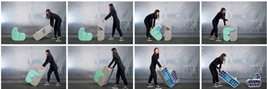
Fig. 2: Human interaction: The process of assembly, disassembly, and lifting of the concrete element through rotational interlocking and manipulated center of mass.
