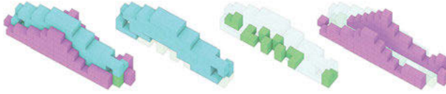
Fig. 11: Assembly environment setup parts. From left to right: Assembly Environment Setup, 2SL-Engagement: hddhddh, Support Blocks, Fixation Blocks.
