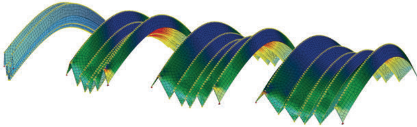
Fig. 7: FE simulation of sample from Fig. 1 (tension and compression from active bending in blue and red, respectively).
