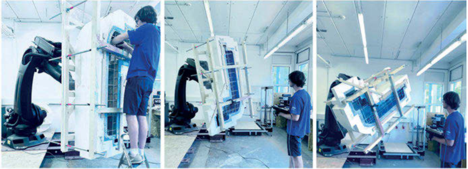
Fig. 9: Robotic sequential casting (RotoForm) of 1:1 hollow concrete element. Left: adding the calculated amount of casting material to the formwork. Right: the robotic arm rotates the formwork to distribute the material along the desired trajectory.
