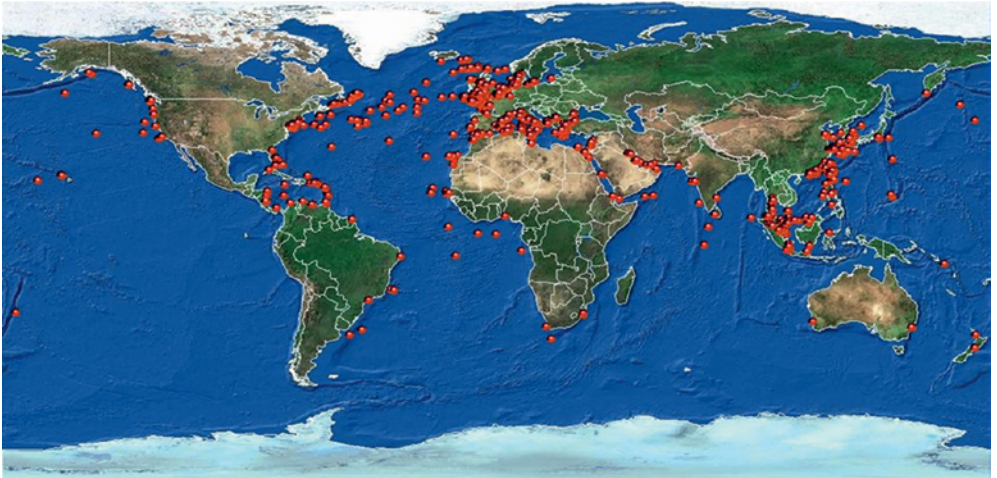
FIGURE 5 This distribution of 2,162 cable faults was recorded between 1959 and 2008, a period that covers the last of the telegraphic cables, all coaxial cables and modern fibre-optic systems, the latter coming to prominence in the late 1980s. Most faults occurred in the shallow (< 200 m deep) seas around Europe, SE Asia and eastern seaboard of North America and reflect the intense fishing and shipping activity of those regions. Faults across the North Atlantic Ocean in part result from the failure of old telegraphic cables due to abrasion and component failure. For the rest of the ABNJ, cable faults are presently on average 4 per annum worldwide. 116 SOURCE: TE SUBCOM, WHICH GRANTED PERMISSION FOR USE.
