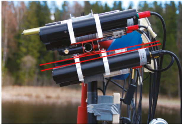
Figure 8. The angle between red lines marking the directions of HyperOCR and RAMSES sensors was measured to be 1.3^\circ from this image.
