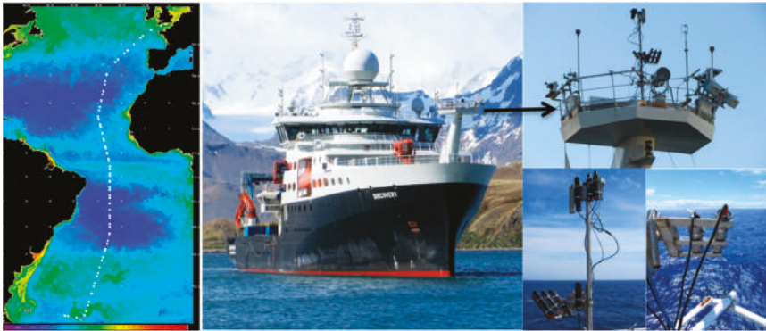
Figure 15. The route of AMT-27 through the Atlantic and the position of the FRM4SOC radiometers on RRS Discovery in operation during AMT-27.
