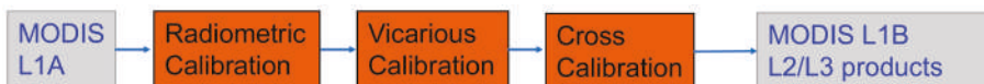
Figure 1. Ocean Biological Processing Group (OBPG) ocean color production process: L1A is the formatted raw instrument data. L1B is the calibrated radiance. L2/L3 are the level 2 and 3 ocean color products [8].
