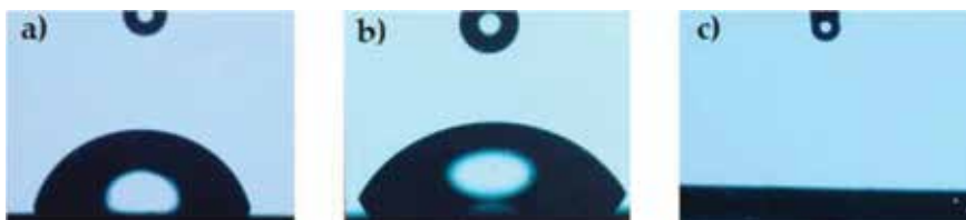
Figure 1. Contact angle between a drop of water and Ti6Al4V bulk material (a), Ti6Al thin film (b) and Ti6Al4V thin film (c).
