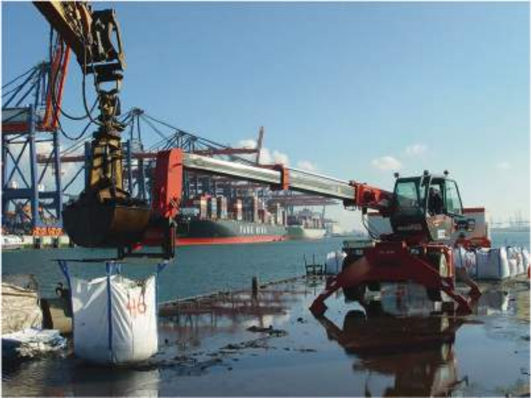
Fig. 8.8 Use of specially designed grab sampler for excavation at the Maasvlakte excavation showing a large bag being filled with sediment sampled from a sand layer at 18 m below sea level. Photo by Dimitri Schiltmans, BOOR
