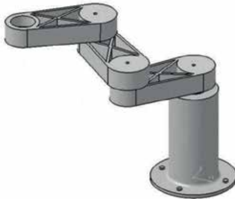
Fig. 4. The considered generalised planar robot with three links and horizontal work plane. Referring to Figs. 5 and 6 the next notations are also employed:
