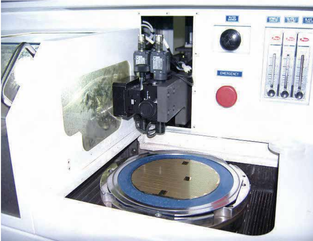
Fig. 5. Photo of automatic wafer dicing machine
