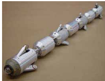
Fig. 10. Pipeline Explorer from NREC (reproduced from http://www.rec.ri.cmu.edu/projects/explorer )
