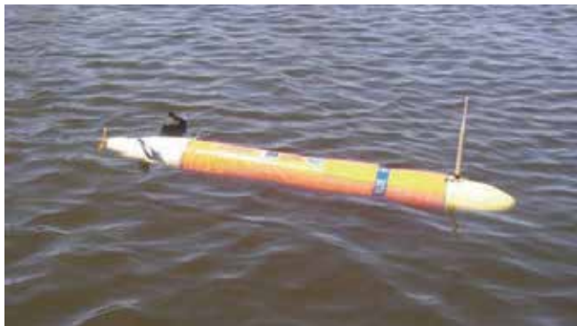
Fig. 1. Light Autonomous Underwater Vehicle (LAUV) designed and built at University of Porto.
