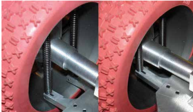
Fig. 16. Close view of springs in passive suspension of Wheeler during riding over obstacle
