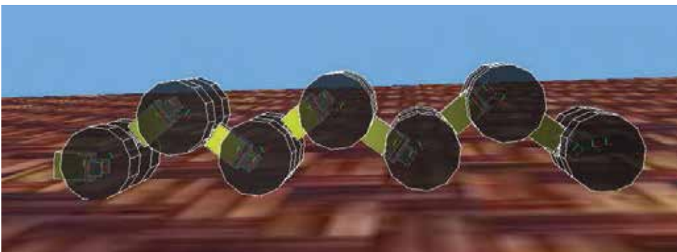
Fig. 14. Zigzag configuration of Wheeler for working in pipes, shafts and low ceiling environments.
