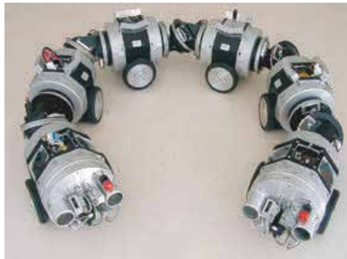
Fig. 5. MAKRO plus robot for sewer inspection (reproduced from Streich & Adria, 2004)
