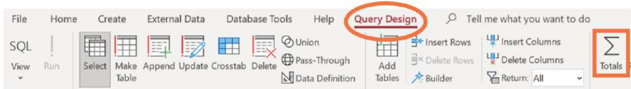
Figure 14.13 The Totals tool is found in the Show/Hide command group when you are designing a query. (Used with permission from Microsoft)
