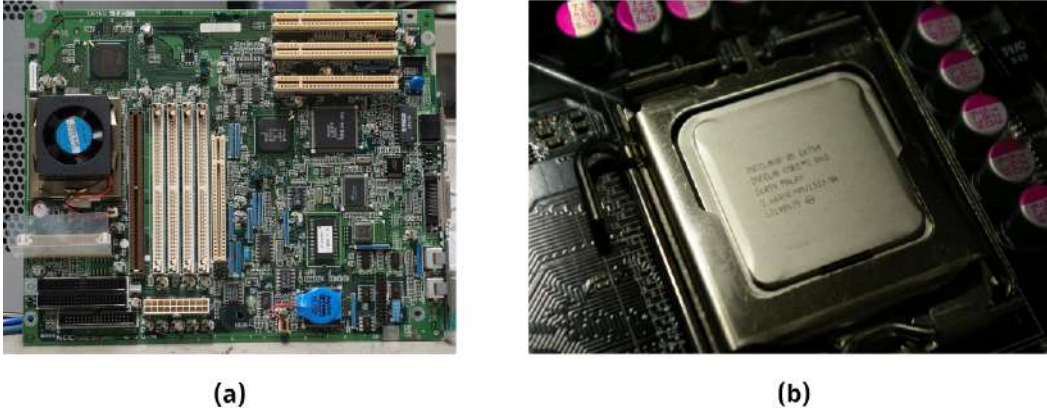
Figure 1.20 Two essential components of a computer's inner workings are (a) the motherboard and (b) the CPU's microprocessor. (credit a: modification of "Green Motherboard" by Pixabay/Pexels, CC0; credit b: modification of "Intel Core 2 Duo E6750" by Nao Iizuka/Flickr, CC BY 2.0)
