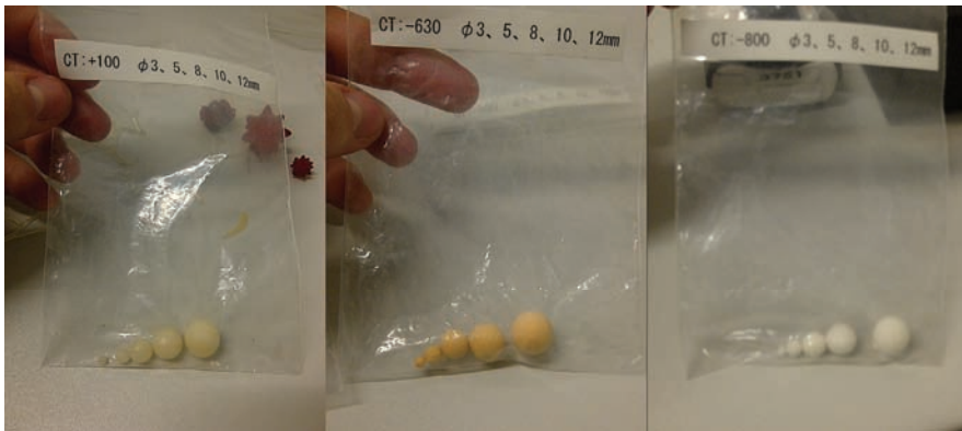
Figure 2. Artificial nodules with diameters of 3, 5, 8, 10 and 12 mm in 3 densities (from left to right solid +100, subsolid -630 and -800).
