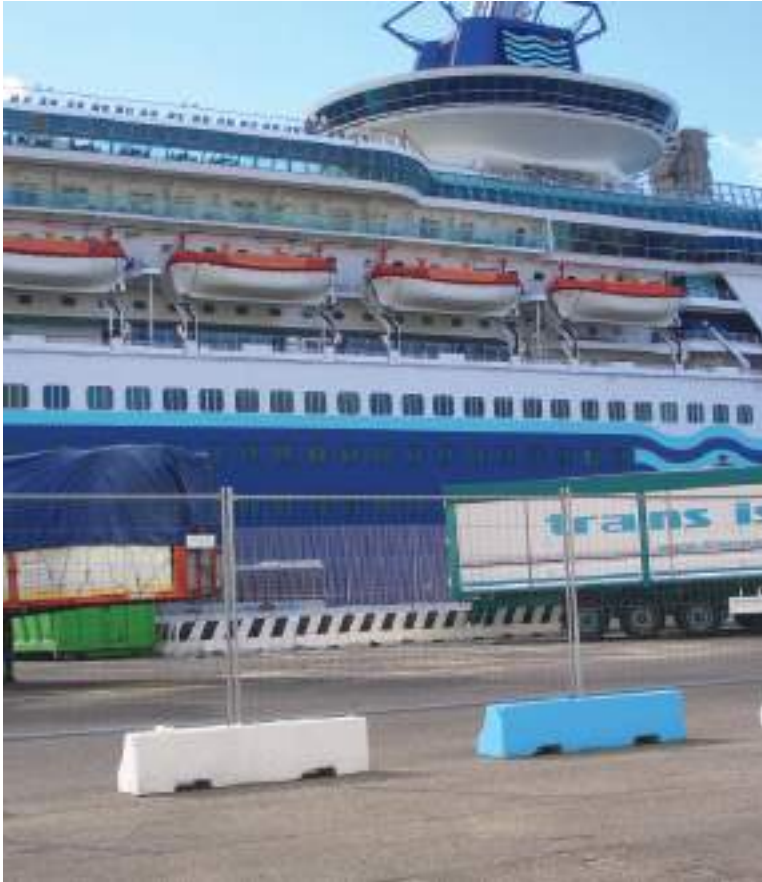
Plate 82 Large passenger vessel with its lifeboats doubling up as tenders to transfer passengers when the ship is at anchor. The tenders have a high capacity 450 persons and form part of the ship's certificated life-saving appliances.
