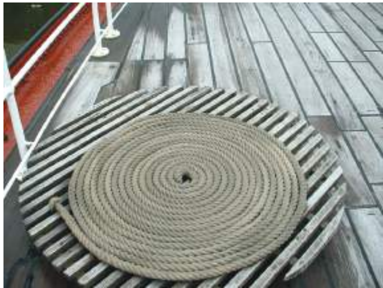
Plate 23 A short manila rope is seen in a 'cheese' on a deck grate. The 'cheese' commenced from the centre, being the basis for the coil which would form on top where any additional length of rope would be coiled right-handed, into a ready-to-use tight coil.
