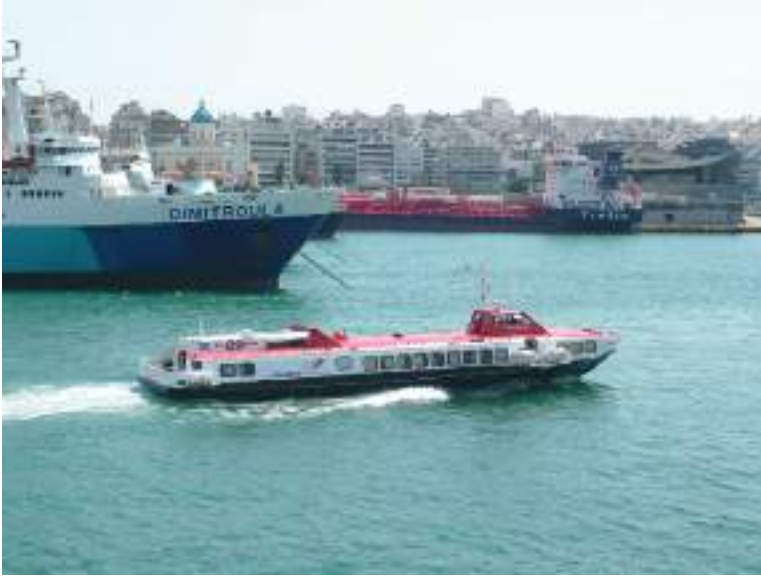
Plate 255 The hydrofoil Flying Dolphin 29 operating with Hellenic Seaways, seen in the displacement mode inside harbour limits of Piraeus. Hydrofoils operate in a non-displacement mode on the plane at high speed in suitable sea conditions (see Plate 7).
