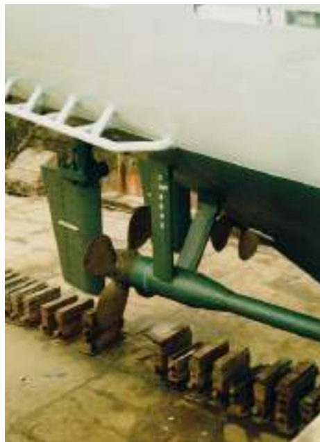
Plate 223 Structural support for twin screw/twin rudder vessel, seen in drydock where each tail end shaft is supported by 'A' frame struts extending from each quarter of the hull.
