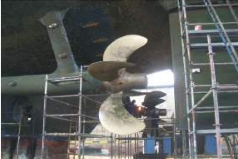
Plate 222 Propeller and spade rudder arrangement of a twin-screw vessel, exposed in dry dock, prior to undergoing maintenance.
