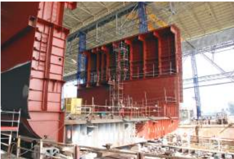
Plate 43 Modern construction of dry cargo vessel in way of double bottom and lower tank sides. The prefabricated section is seen in the enclosed confines of a covered assembly area of a shipyard building complex.
