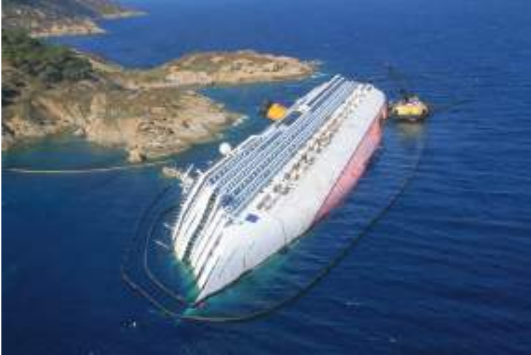
Plate 176 The wreck of the passenger vessel Costa Concordia seen during the period of salvage with anti-pollution oil booms set around the hull. (Source: Shuttlestock.)
