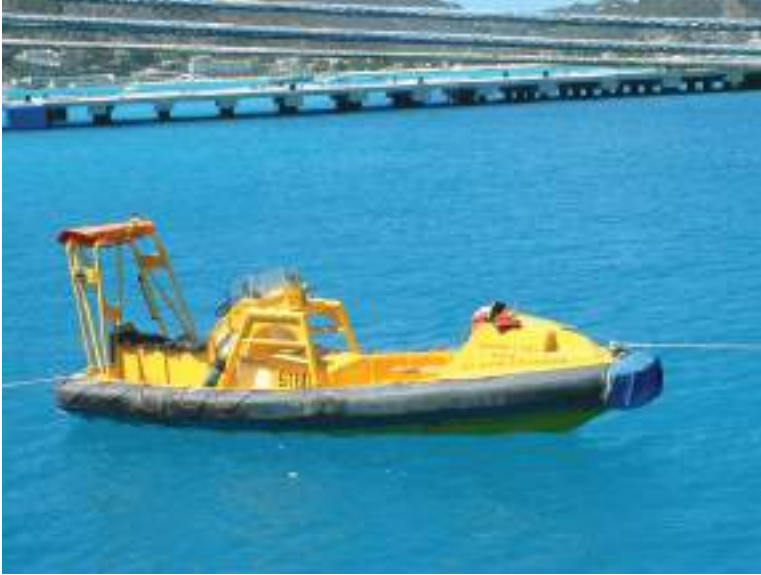
Plate 115 A semi-rigid fast rescue craft as fitted to the passenger ship Explorer of the Seas . It is a requirement that passenger vessels carry a rescue boat on either side of the vessel.
