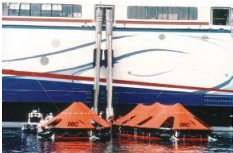
Plate 106 Double chutes deployed with life rafts at the waterside. Example configuration of MEC system as manufactured and produced by Dunlop/Beaufort, Canada.
