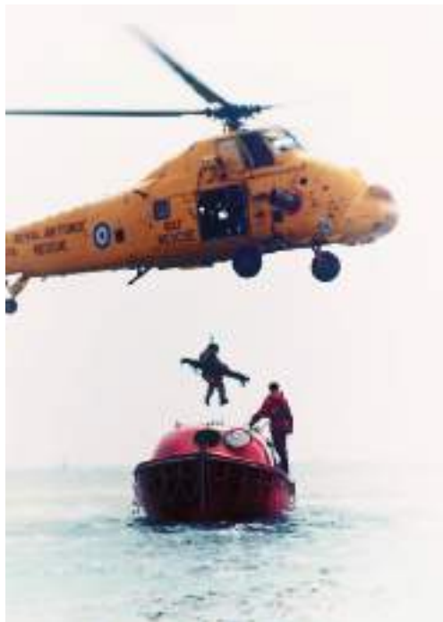
Plate 179 Wessex Mk4 SAR helicopter in operation with the RAF engages in stretcher casualty rescue from a totally enclosed lifeboat at the surface. This type of aircraft has been phased out around the United Kingdom, but continues to operate in other areas of the world.
