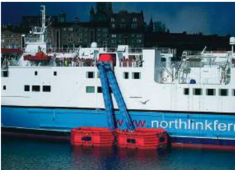
Plate 108 Evacuation drill being conducted with the RFD Marine-Arc marine evacuation system. Two chutes, two life rafts being deployed on the portside of a North Sea ferry.
