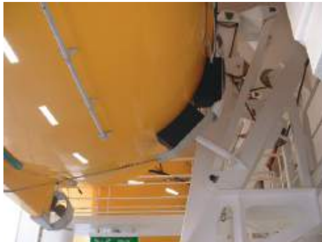
Plate 76 Boat's skate set inside of the boat's hull manufactured in hard rubber and metal strapped. Seen fitting the curve of the boat with the securing wire passing under the keel. The bilge grab rail and retro-reflective tape are fitted to the boat's underside.
