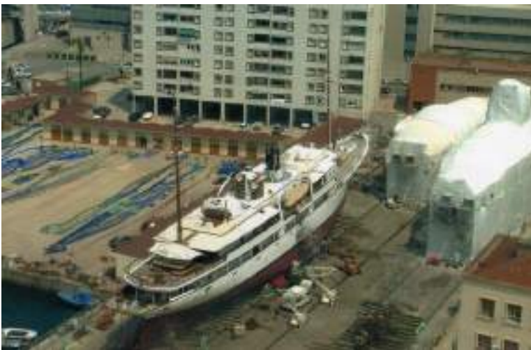
Plate 184 Large yacht drawn onto a slip for maintenance. Slips vary in size and are also used for building prefabricated new constructions. However, slips are generally employed for the smaller coastal craft, fishing vessels, large yachts and the like.
