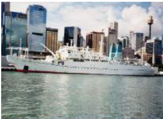
Plate 3 The cable vessel Pacific Guardian lies starboard side to the berth. The type of ship is distinctive, with cable fitments at the bow and the stern positions.
