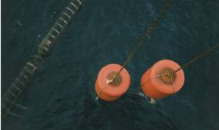
Plate 268 Example pick-up buoys in use next to a floating pipeline from a floating storage unit (FSU).
