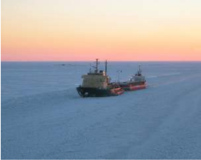
Plate 168 A Finnish ice-breaker engages in close-proximity towing to assist a vessel in the Baltic Sea ice conditions.
