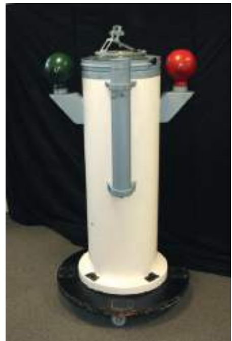
Plate 141 Modern binnacle shown without ‘helmet’ in position, but with azimuth circle in position on the top of the compass bowl.
