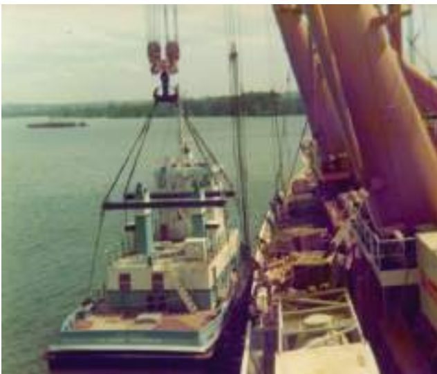
Plate 29 Ram's horn hook engaged with Stülcken mast. Seen with heavy lift being lifted on board.
