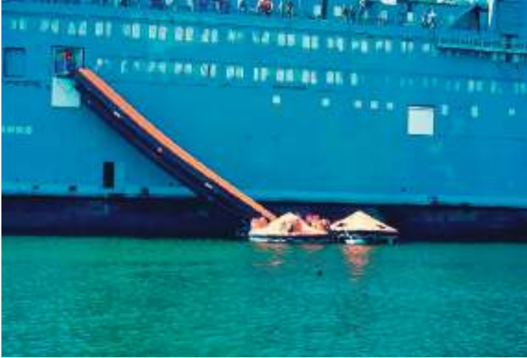
Plate 105 Viking MES deployed showing the slide to the surface. A large 45-man life raft is secured alongside the boarding platform.
