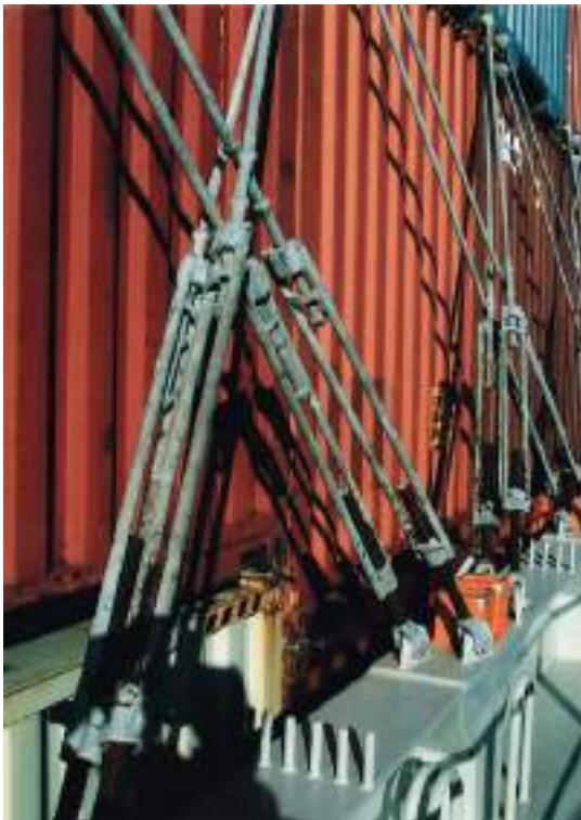
Plate 71 Container lashing bars, seen secured from the pontoon to the second tier of deck containers.
