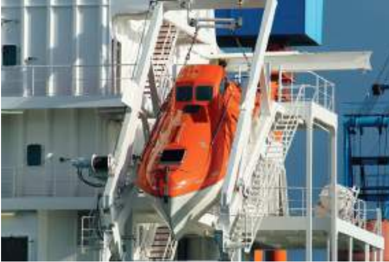
Plate 88 Free-fall lifeboat stowed at the aft end launch position. (Source: Shutterstock.)
