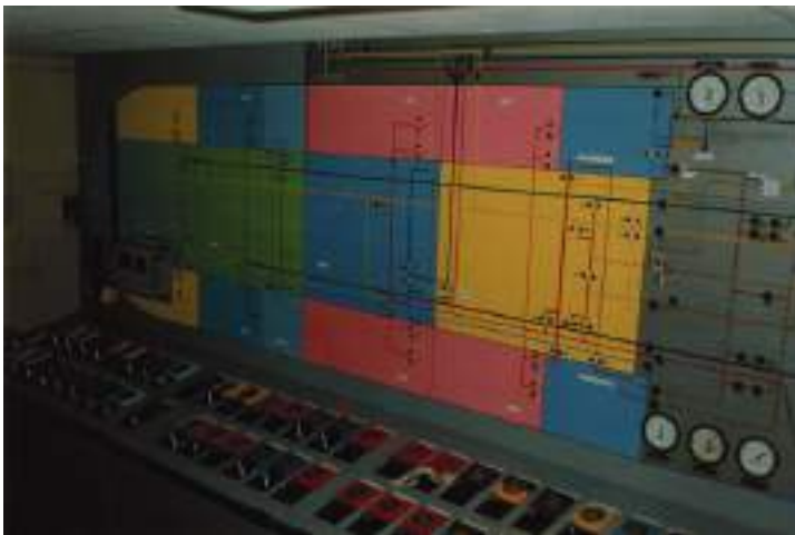
Plate 258 Mimic diagram for tanker pipeline systems seen in a cargo control room of a tanker vessel.
