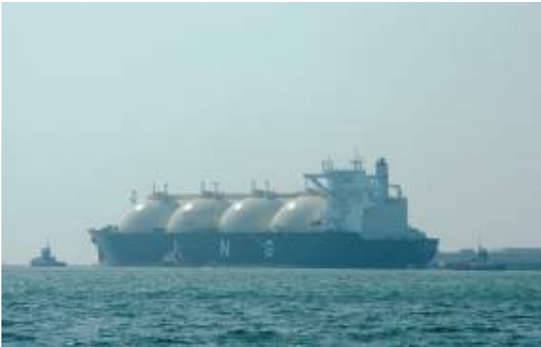
Plate 270 Large Gas carrier seen manoeuvring with tugs in attendance. The four prominent spherical tank 'domes' clearly identified above the uppermost continuous deck. Fully refrigerated spherical LNG tank, the protective steel dome protects the primary barrier above the upper deck. (No secondary barrier.) Double hull construction required in way of all cargo tank spaces.
