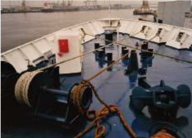
Plate 16 Foredeck of a passenger vehicle ferry with split windlass arrangement incorporating a powered warping drum. An additional mooring is on the end rope drum. The spare stockless anchor is seen strapped to the deck on the centre line.
