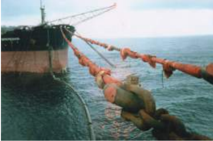
Plate 262 Tanker moorings and floating pipeline seen connected to a floating storage unit (FSU).
