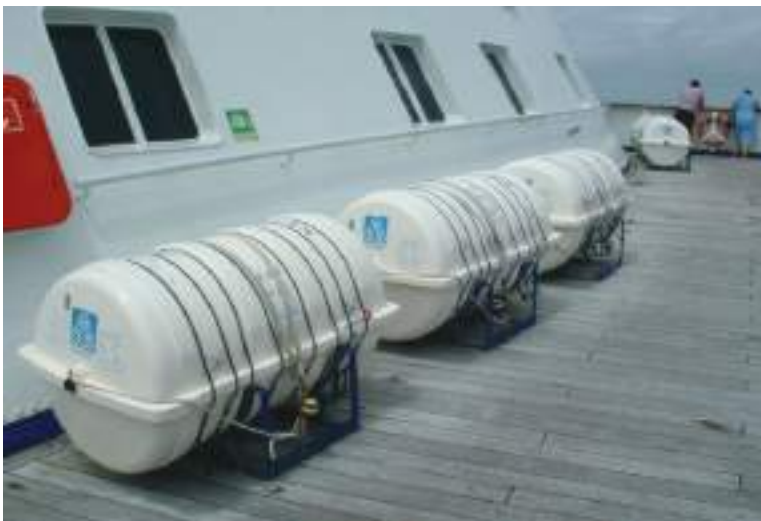
Plate 99 Davit-launched inflatable life rafts stowed either side of the fore and aft line on a passenger cruise ship. Davits (not shown) fitted either side on the foredeck. Each raft is secured by a hydrostatic release system and can be launched as a throw-over inflatable should the davit be indisposed.
