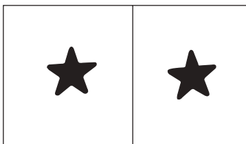
Figure 11.5 Images of true and reflected stars, showing side error, when sextant at zero.
