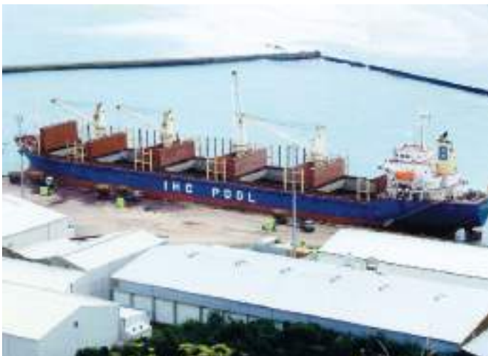
Plate 44 Bulk carrier Mount Travers IMO 9263772, seen loading logs in Gisborne, New Zealand. The five-hatch ship is seen with all folding hydraulic hatch covers opened and in the upright stowed positions. All four pedestal cranes are topped and working a cargo of logs.
