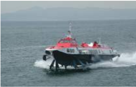
Plate 7 A high-speed hydrofoil seen at sea operating off the Greek coastline. The lower hull supporting struts are set either side to the bow and quarter regions of the hull. Tyre fender supports are also seen either side in the shoulder and off the port quarter. Prominent bow flare is often a feature of such craft often engaged on the 'plane' in open waters operating in excess of 45 knots.
