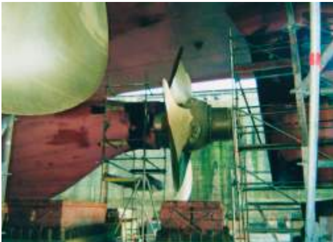
Plate 221 Controllable pitch propeller of a twin-screw ship seen exposed in drydock. The picture shows the blades bolted to the hub by four bolts per blade. This allows each blade to be individually removed/replaced for maintenance, if required.
