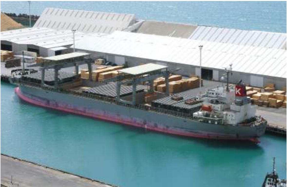
Plate 55 Package timber being loaded by means of ship's travelling gantry crane aboard the Pan Pac Spirit (IMO 9186780) seen lying starboard side to the timber berth in Napier, New Zealand.
