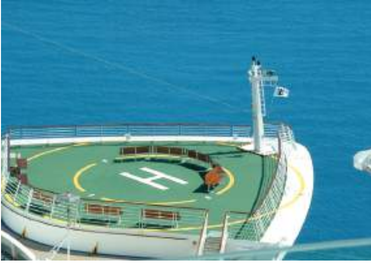
Plate 200 Helicopter operational area marked on the upper foredeck of a large passenger vessel. The obstructions of the fore stay and seating benches would be cleared prior to aircraft engagement.
