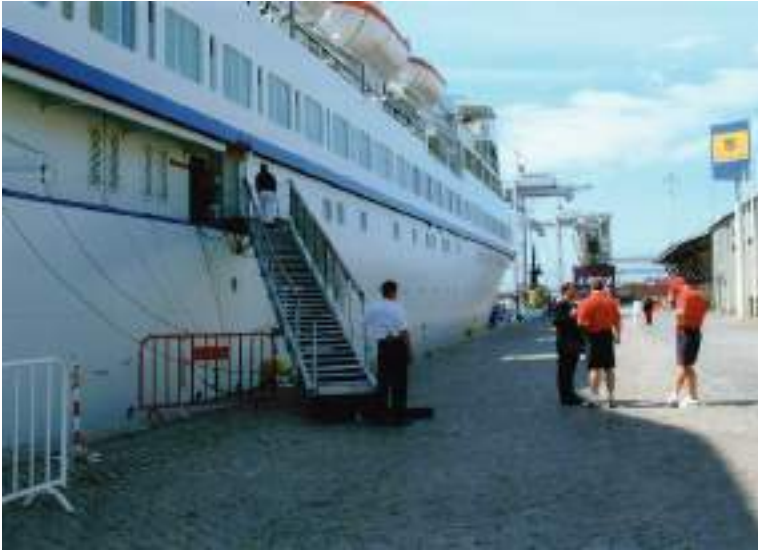
Plate 134 Accommodation ladder seen rigged with stanchions, manropes and gangway net landed to the quay with the bottom roller clear of obstructions.
