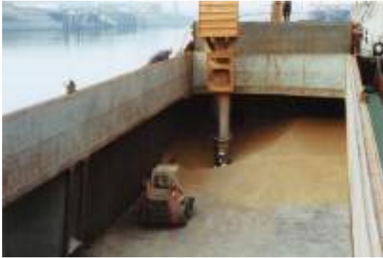
Plate 48 Grain elevator and tractor engaged in clearing the remnants of bulk grain cargo.
