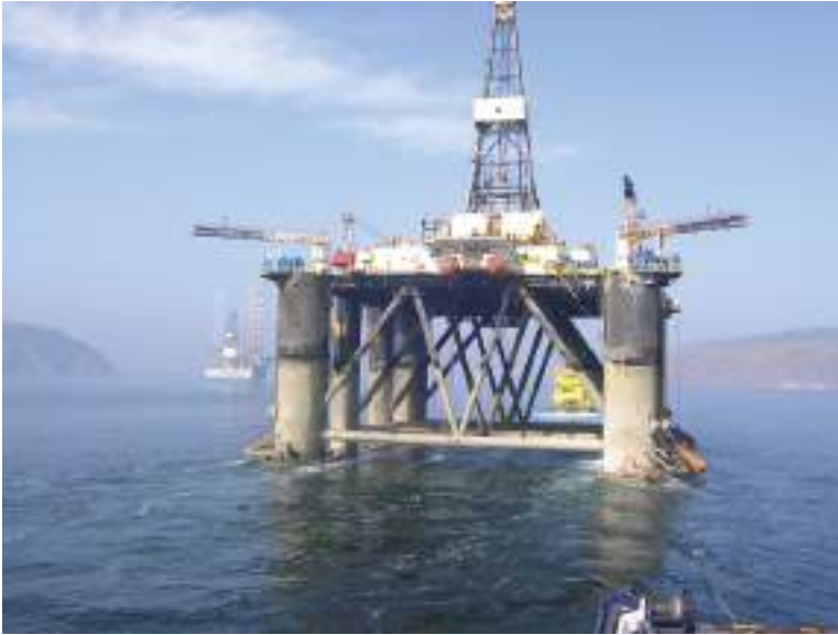
Plate 251 The SEDCO 704 offshore installation, seen under tow by the Tug/supply vessel Vidar Viking , as seen from the brake tug.
