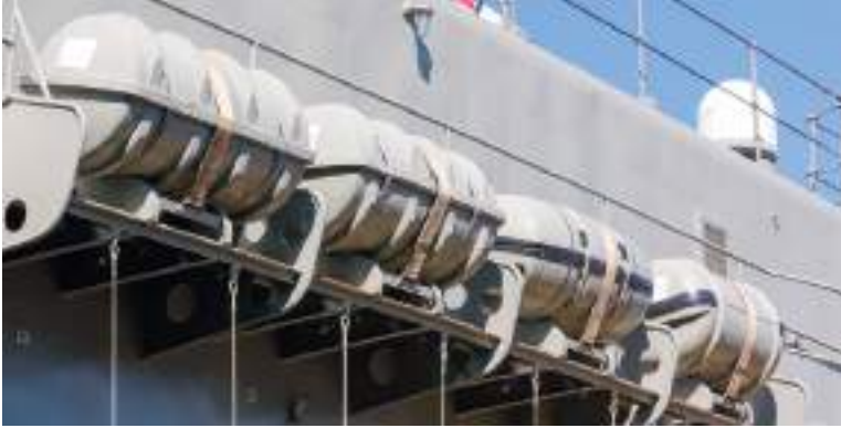
Plate 94 Racked inflatable life rafts stowed aboard a passenger cruise liner. (Source: Shutterstock.)
