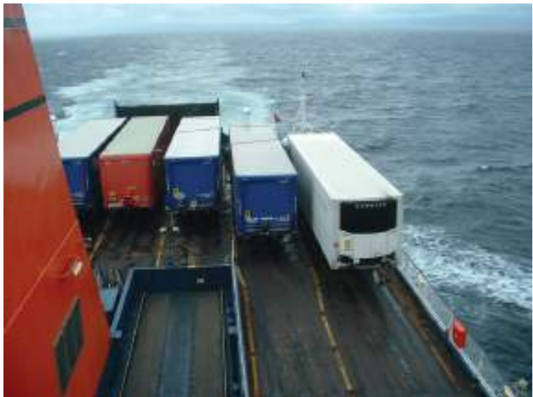
Plate 214 Ro-ro vehicle open upper deck. Drop units secured to the aft part of the upper deck. Cargo units carrying hazardous goods are often stowed in such a position to cause any harmful vapour or smoke to be blown overside in the event of leakage or fire.
