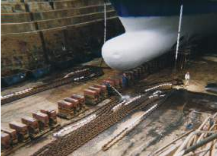
Plate 183 The bulbous bow of a ship seen on the keel blocks of a typical graving dock. Attention is drawn to the port and starboard anchor cables seen ranged on the bottom of the dock.
