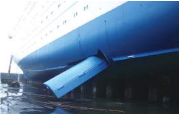
Plate 234 Fin stabilizer unit turned out and exposed on a vessel in drydock.
