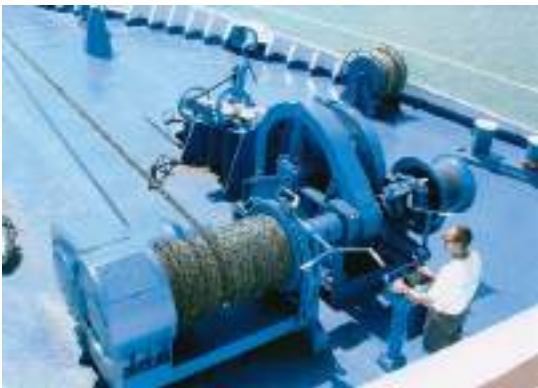
Plate 13 An electric windlass and combined mooring winch. The compressor, bow stopper, is seen over the anchor cable, which leads to the gypsy.
