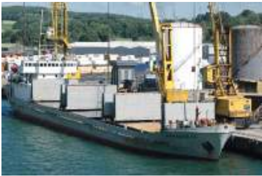
Plate 50 Fully open hydraulic hatch tops seen aboard the Baltiyskiy-110 , lying alongside the berth at Warrenpoint Northern Ireland, port side to. Cargo operations are engaged with use of shoreside mobile cranes.
