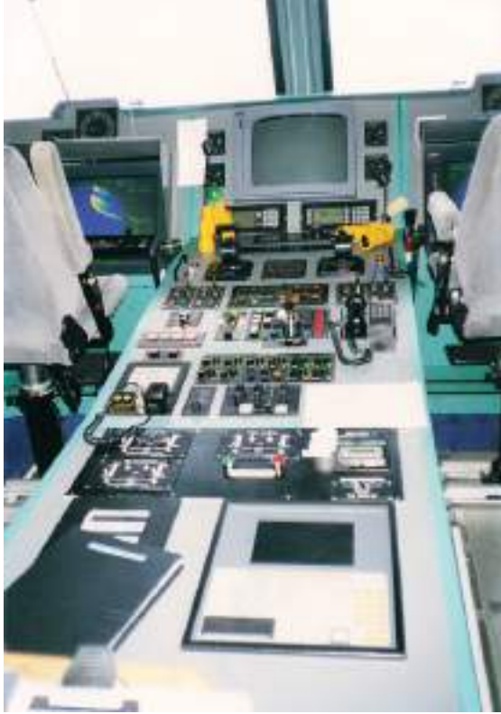
Plate 217 Central bridge control console set into the integrated navigation bridge of a modern high-speed craft.
