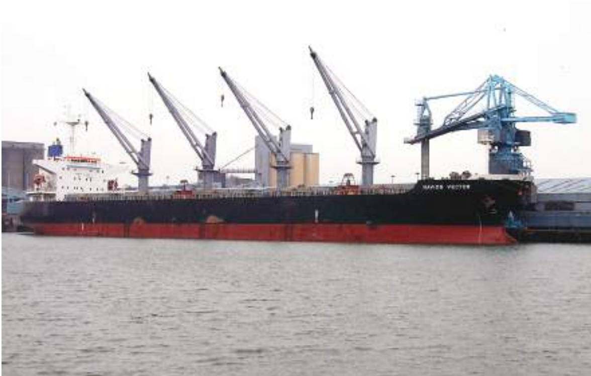
Plate 31 The bulk carrier 'Navios Vector'. Fitted with pedestal deck cranes, all topped and turned outboard to make way to allow a ship loading unit access to cargo holds.
