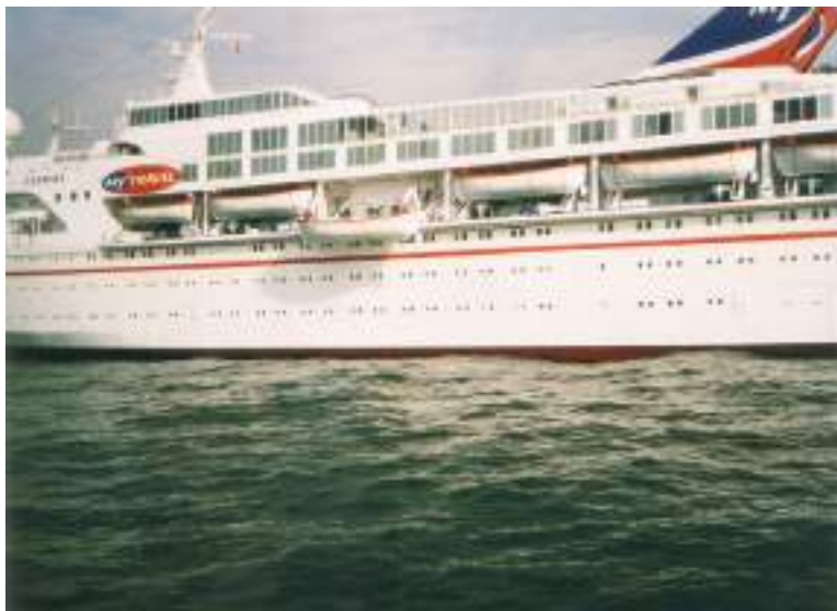
Plate 89 No. 6, open lifeboat turned out and ready for launch down the portside of a passenger cruise liner.
