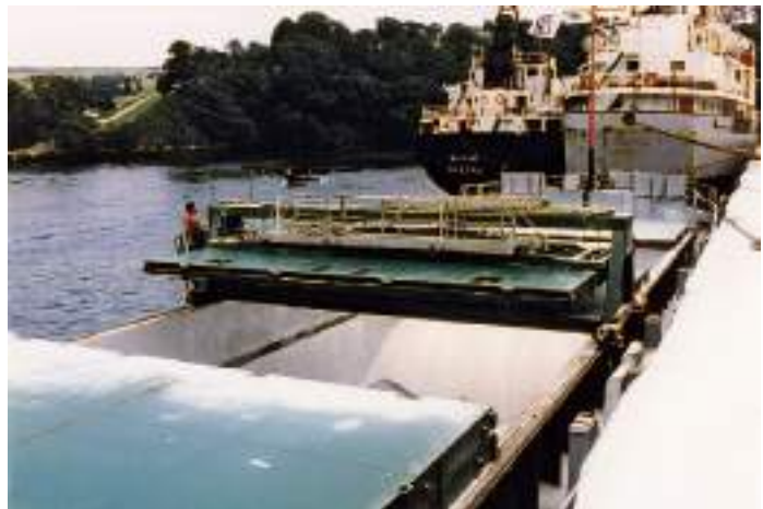
Plate 45 Stacked steel hatch covers aboard a modern coastal vessel. The ship is fitted with its own travelling mini-gantry crane.
