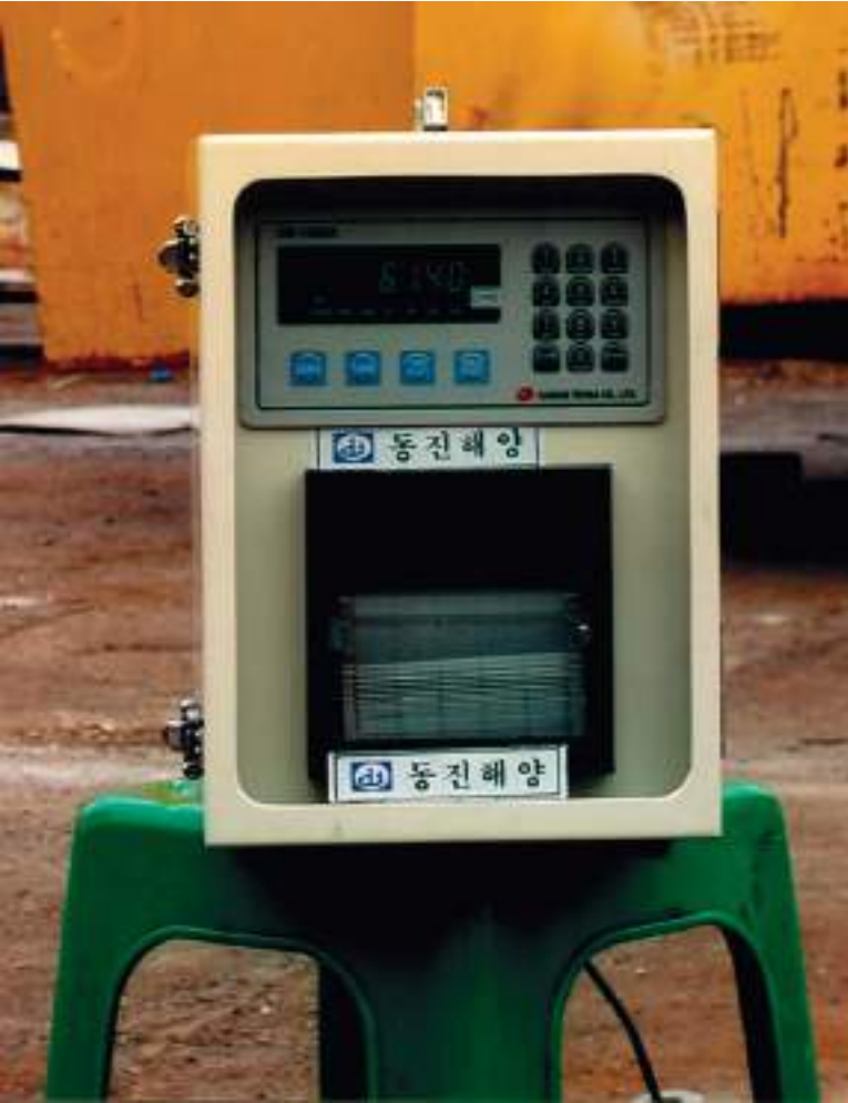
Plate 33 Example of a digital load cell as employed in modern shipyards.
