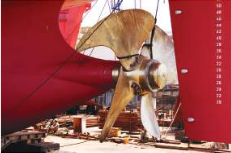
Plate 219 Arrangement of controllable pitch propeller and mariner rudder blade seen exposed in dry dock.
