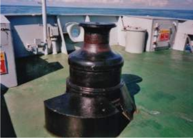
Plate 237 Single (old man) roller lead. Such examples can be motorized to work as a capstan.
