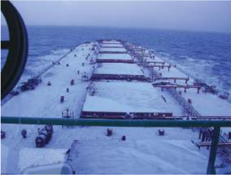
Plate 74 The large bulk carrier Berge Norde seen at sea with an ice-covered foredeck. The side moving steel hatches have a dominant position, seen closed and battered down for sea passage across the North Atlantic.
