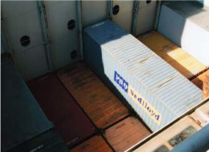
Plate 70 Twenty- and forty-foot container units stowed in the cell guides aboard a large container vessel.
