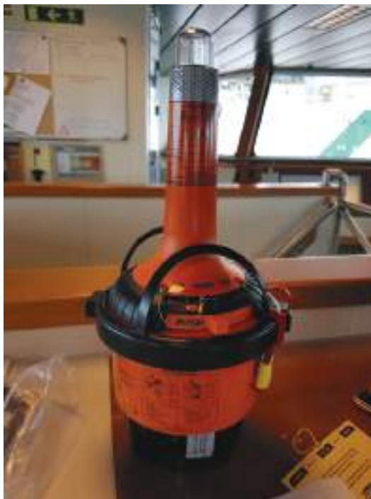
Plate 123 The TRON 40VDR EPIRB, manufactured by 'Jotron', stores the data from the VDR and can be recovered in addition to the 'Black Box'.
