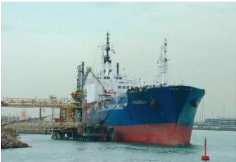
Plate 274 The Annabella gas carrier seen alongside a river berth discharging the cargo by the flexible shore link.
