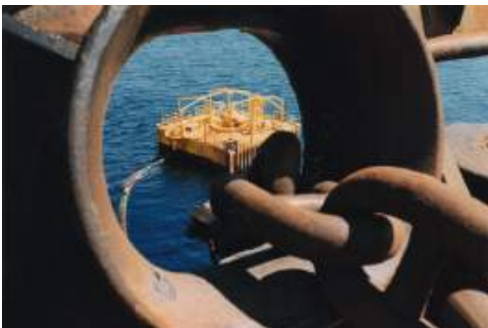
Plate 264 Single point mooring buoy as seen through chain mooring pipe lead. (Floating oil pipe is also seen at surface, which would be led aft to connect with manifold).
