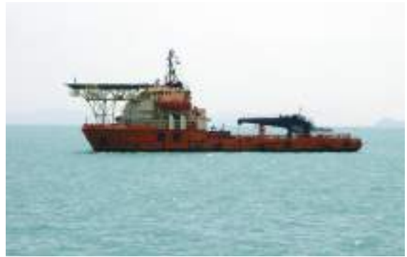
Plate 8 Offshore support vessel Toisa Mariner . Seen with prominent heli-landing pad above the bridge structure and heavy-duty deck crane aft. Large aft deck permits the carriage of essential supplies to offshore installations.
