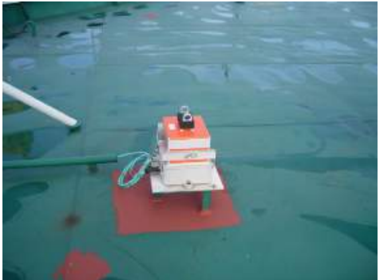
Plate 148 Example of a voyage data recorder, mounted to an upper exposed deck area.
