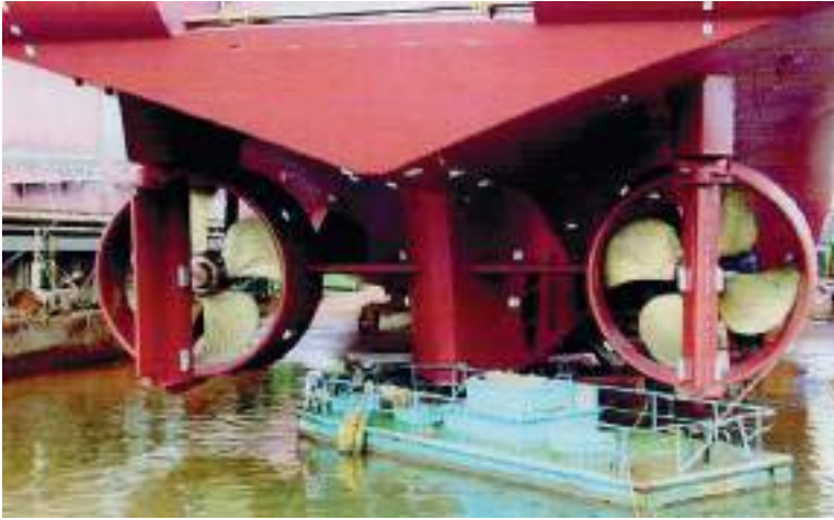
Plate 227 Twin ducted propellers with twin rudders, set either side of a centre line skeg which is fitted with fore and aft stern thruster unit.
