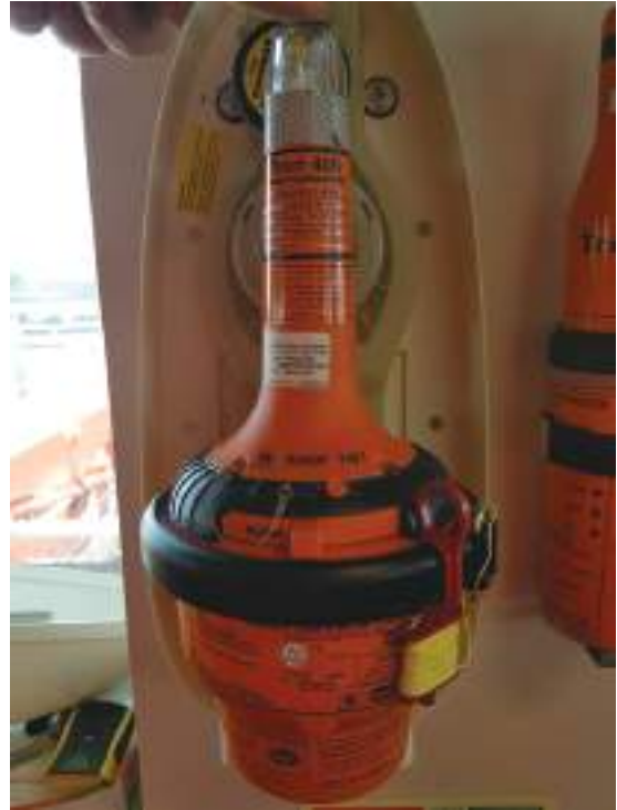
Plate 121 Bulkhead mounted Jotron 40S EPIRB exposed with protective cover open, reveals the Hammar hydrostatic release unit, set behind the upper region of the beacon.
