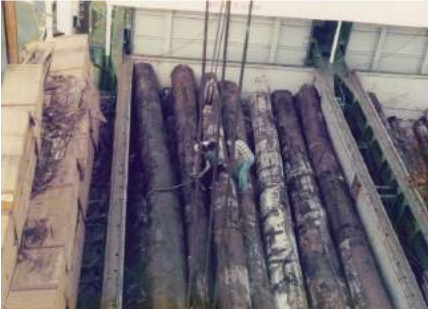
Plate 54 Logs being loaded up to the hatch coaming by use of wire snotters.
