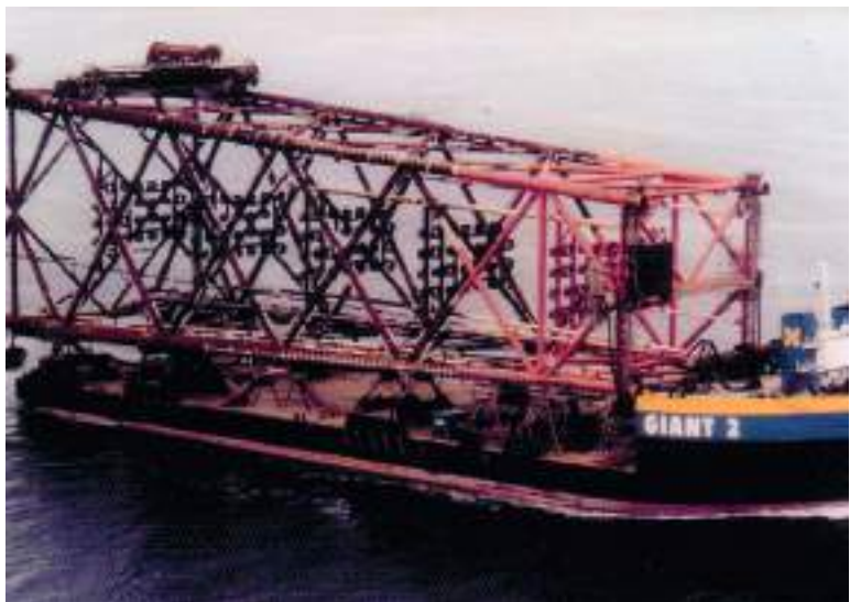
Plate 39 Motorized cargo transport barge Giant 2 . Seen underway and making way with a project cargo, an offshore jacket construction welded on to its deck.
