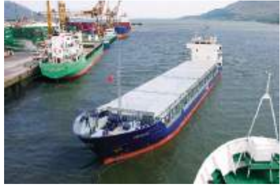
Plate 49 The coastal vessel Uranus approaches the berth with MacGregor steel hatch tops fully closed.
