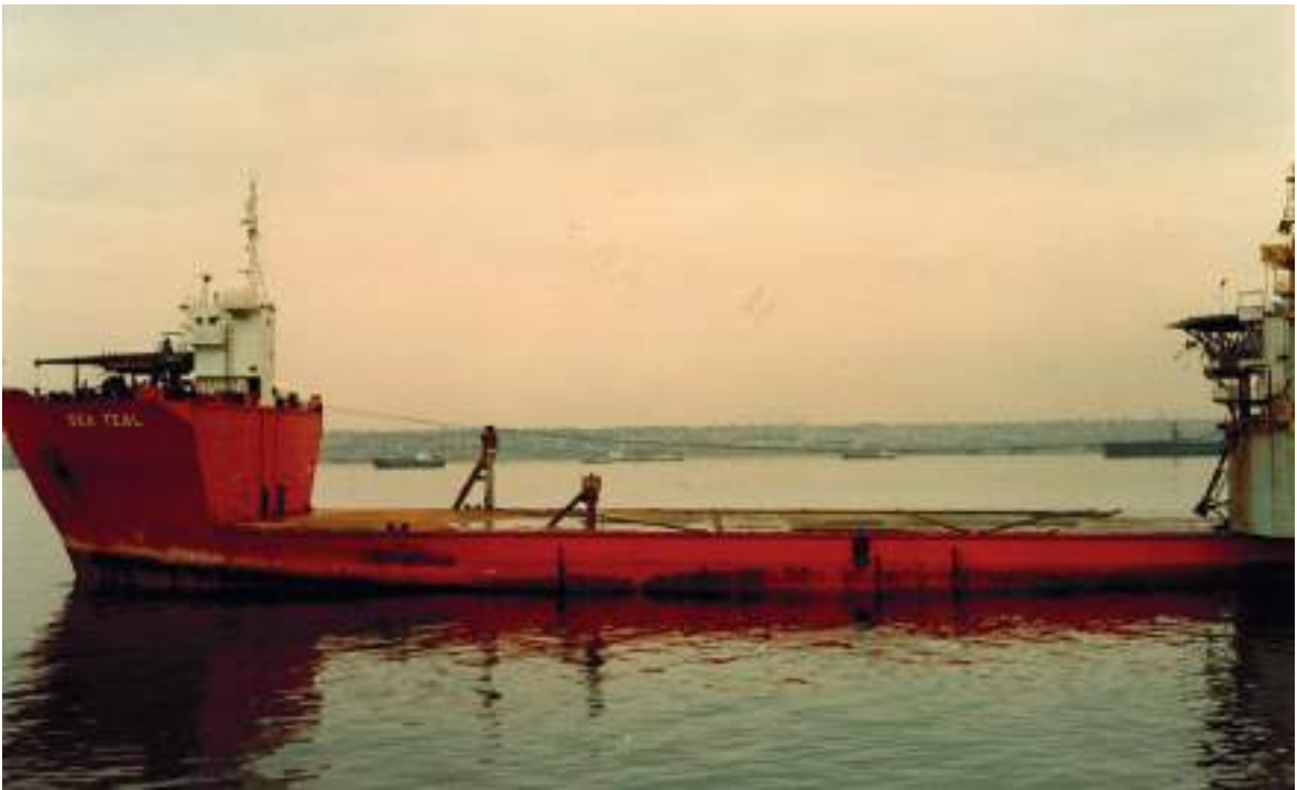
Plate 36 The heavy lift ship Sea Teal seen in light condition with empty tanks with the upper deck exposed. Once the tanks are filled the deck is submerged and permits a float-on, float-off operation. In the case of a ship, is the vessel capable of accepting the load. What is the displacement and physical size of the vessel and its deck load density capability. What is the metacentric height ('GM') and what will be the new 'GM' with the load added. General assessment of the ship's stability throughout all stages of the passage. Endurance of the vessel and the effect of burning bunker oil and consuming water. Ballast movement and the ability to trim or list the vessel for the purpose of loading/discharging. Number of crew, experience of the Master, charter rates, and not least the availability of the vessel.
