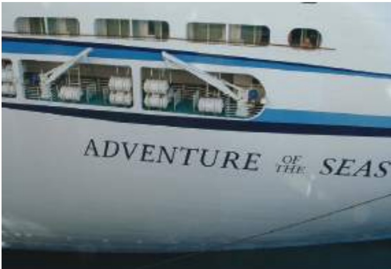
Plate 98 Davit life raft launch station aboard the passenger ship Adventure of the Seas .
