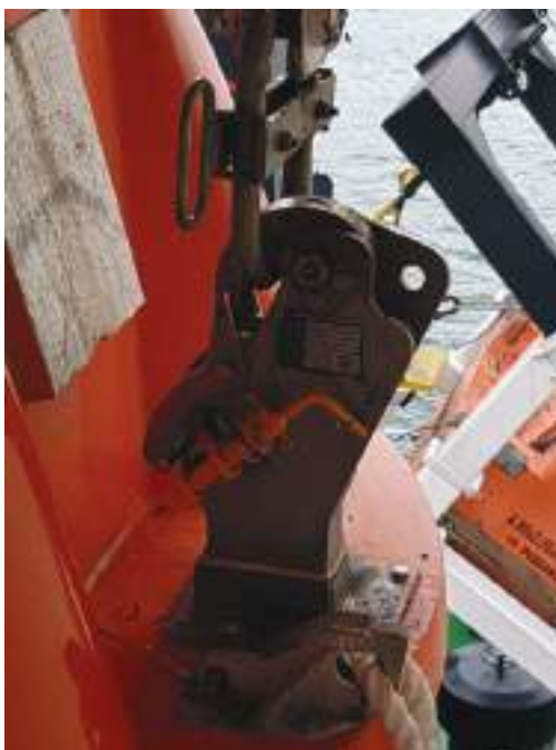
Plate 90 Fall preventative at locking pin, seen in position, prevents release.
