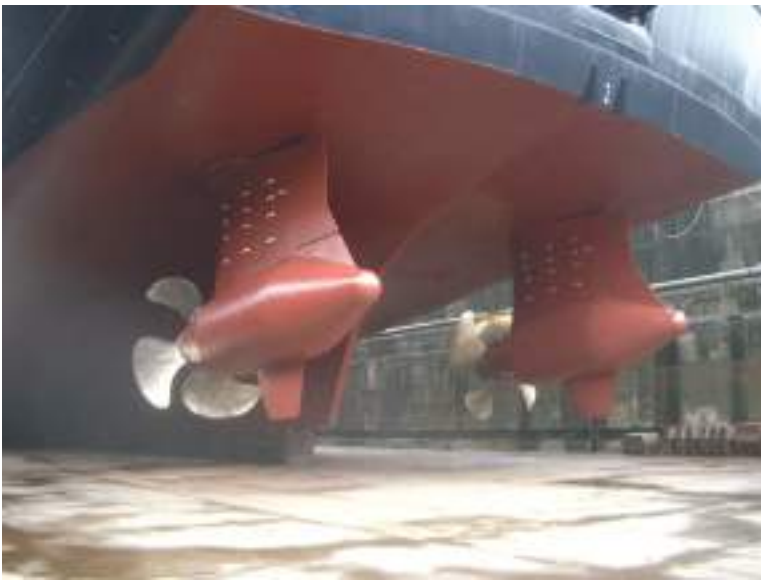
Plate 228 Twin pod propulsion units seen on the passenger vessel Amsterdam exposed in drydock.
