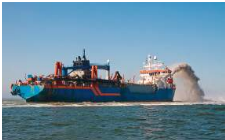
Plate 10 A suction dredger engaged in depositing silt. (Source: Shutterstock.)
