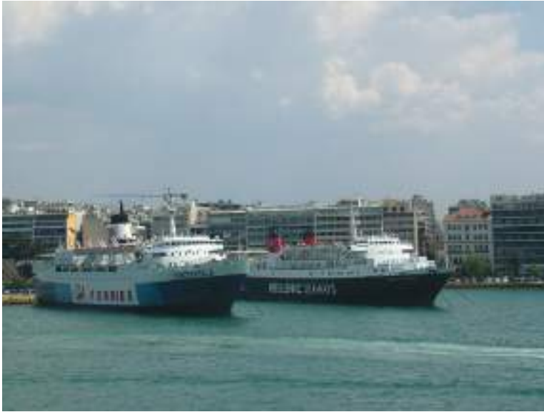
Plate 242 Passenger/vehicle ferries lie stern to quay in Mediterranean moors in the Greek port of Piraeus.
