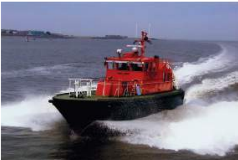
Plate 130b The Liverpool Pilot launch seen at sea under speed. The boat is fitted with deck mounted guard rails and lifebuoys either side of the foredeck. It is equipped with radar and search light mounted to the cabin deck-head.
