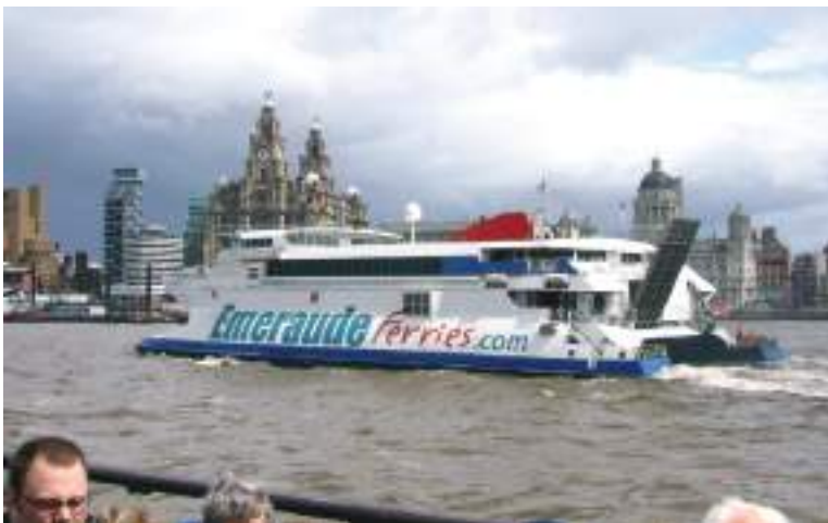
Plate 229 Multi-hull design high-speed ferry operating in the River Mersey. Major changes to hull design have changed many marine aspects, not least ship handling and manoeuvring, but also rescue and survival recovery operations.
