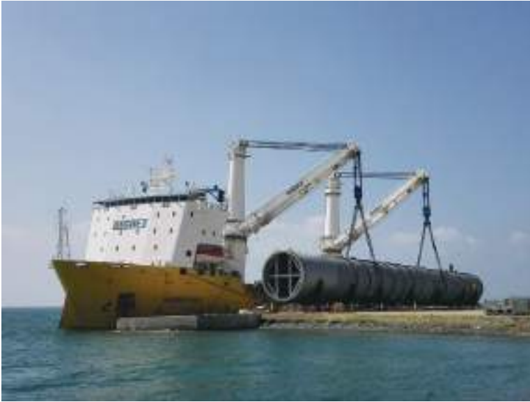
Plate 40 One of Big Lift's designated heavy lift marine transports Happy Sky engages in a tandem lift operation on a long 110m load.
