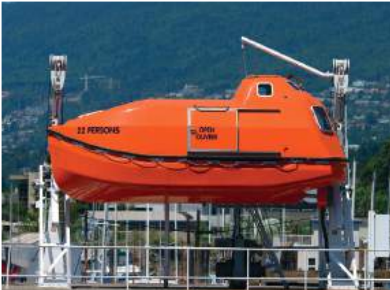
Plate 77 Totally enclosed motor propelled survival craft (TEMPSC) stowed in davit arrangement. Launch control wire clearly seen above the coxswain station. (Source: Shutterstock.)
