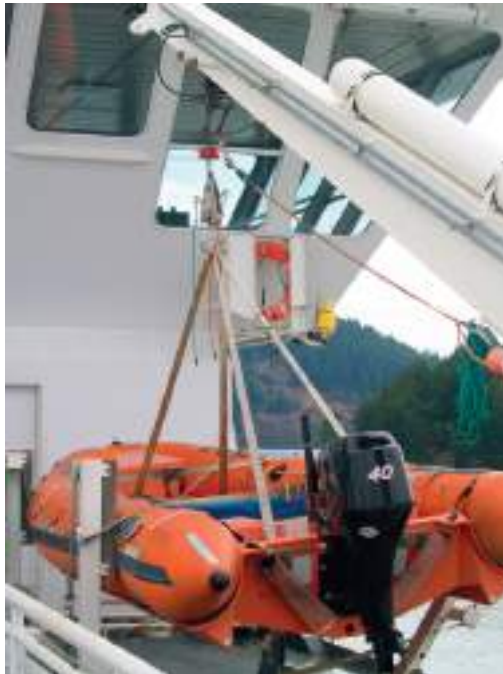
Plate 113 Semi-rigid fast rescue craft held by a four-leg launching bridle under the davit launch system. The system is fitted with quick release and an outboard motor on the transom stern. (Source: Shutterstock.)
