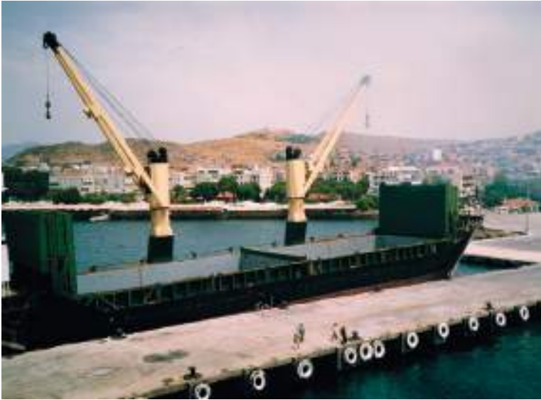
Plate 42 Open hatchway seen exposing the two holds of the Scandi Spirit , with the folding 'M' type hydraulic hatch covers in the fixed open position. Hatches serviced by two port side pedestal cranes.
