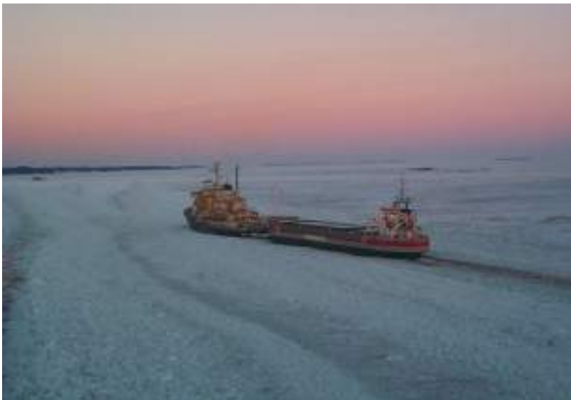
Plate 169 Ice-breaker engages in an escort towing operation to a small coaster in Baltic ice conditions February 2003.
