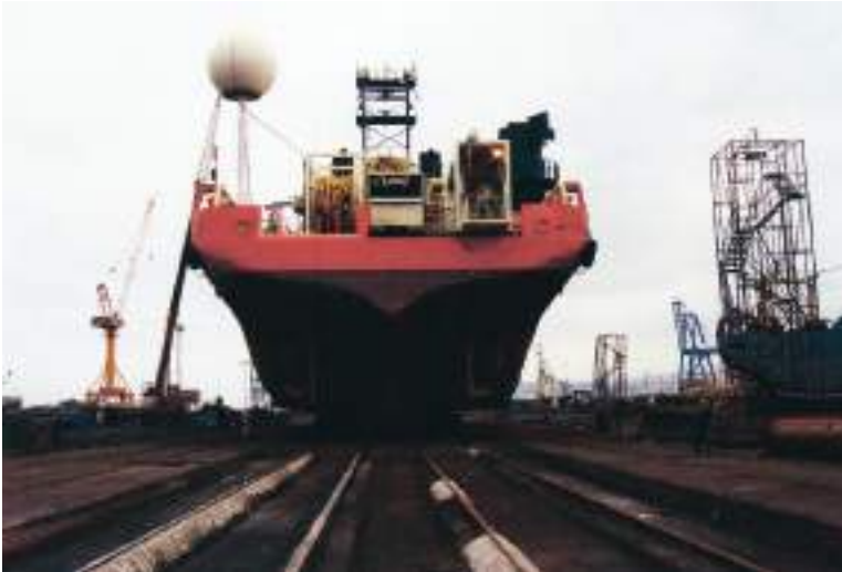
Plate 187 Vessel on the tracks in a dock park after being raised on the synchro-lift. Such a docking principle allows easy access to all parts of the hull for maintenance purposes.
