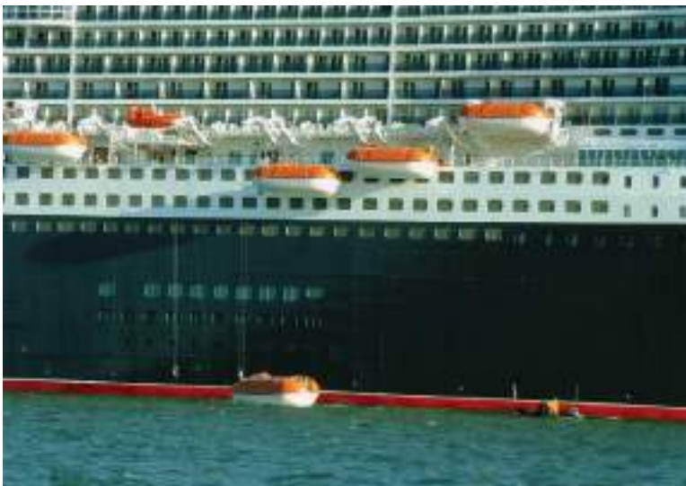
Plate 75 Boat deck and survival craft launching exercise from the Queen Mary 2 while lying portside to in Southampton water. The boats being launched are of the partially enclosed type and a semi-rigid rescue boat is seen at the surface. The starboard rescue boat is also seen stowed in its launching position at the boat deck level.
