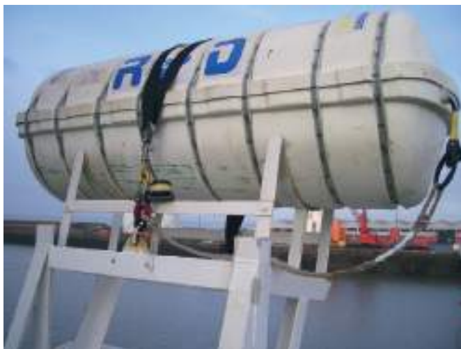
Plate 97 Inflatable RFD life raft contained in GRP container, secured with binding straps in a Stowage/launch cradle and fitted with hydrostatic release unit with painter attached.
