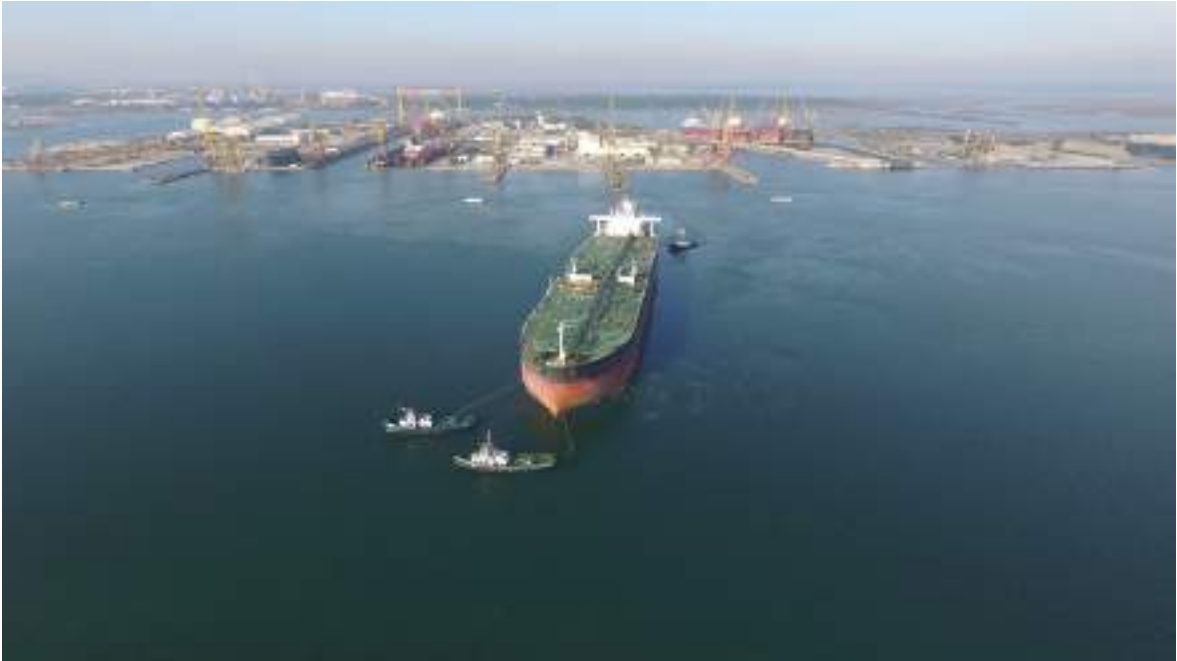
Plate 257 Large crude oil tanker being manoeuvred by three escort tugs prior to entry into the Lisnave shipyard docking complex for routine maintenance.
