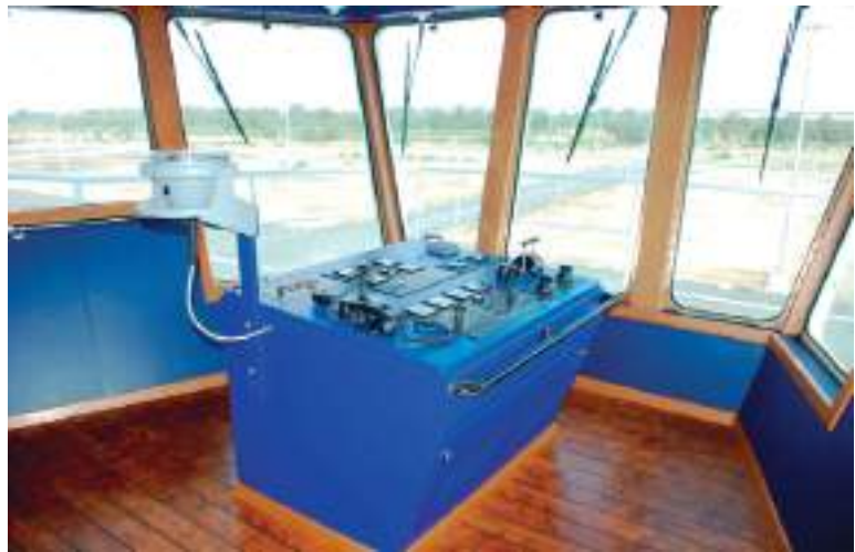
Plate 147 Enclosed bridge wing control console, showing a prominent gyro repeater which can be fitted with a pelorus bearing vane.
