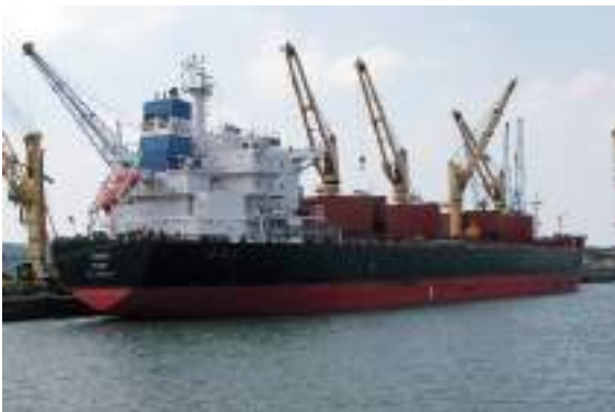
Plate 9 A general cargo vessel working cargo alongside. Fitted with cranes and open steel hatch covers.
