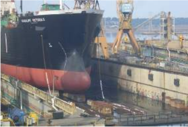
Plate 192 The Guadalupe Victoria II , seen in the Hydrolift complex at Lisnave, Portugal. Hull shown recoated and the ship has both anchor cables ranged on the floor of the platform dry dock.
