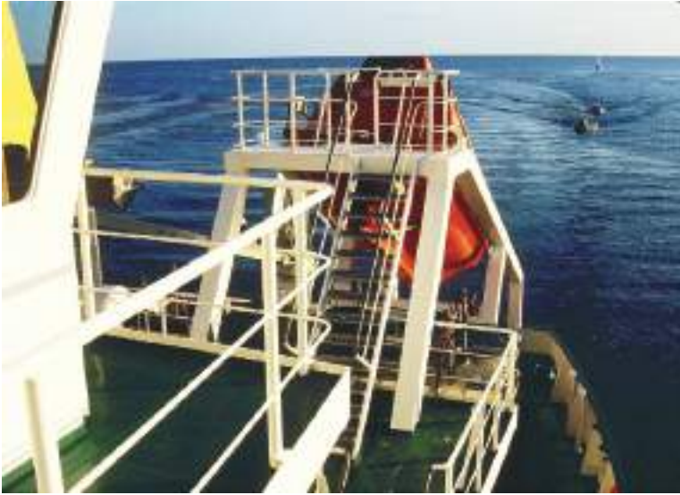
Plate 86 Boarding arrangement and support structure for a totally enclosed free-fall lifeboat situated for over the stern launch from the vessel.
