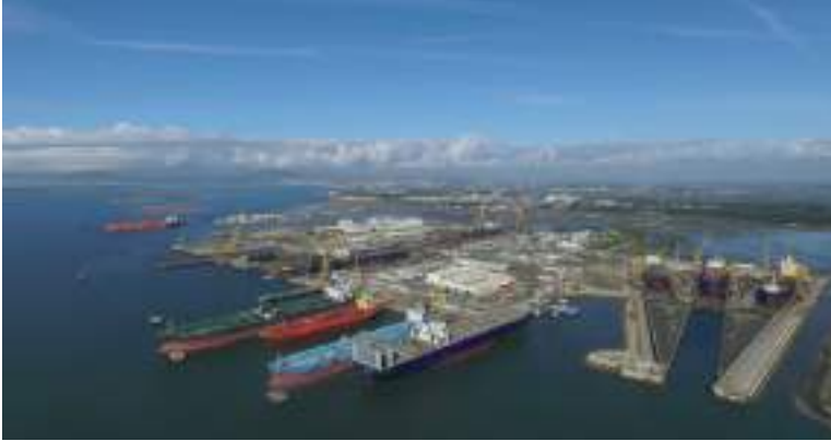
Plate 198 Ariel view of the Hydrolift docking system at the Lisnave, shipyard complex, Portugal. The wet basin is seen drained with the outer caisson open and all three docking platforms occupied by vessels dry docked for routine maintenance.
