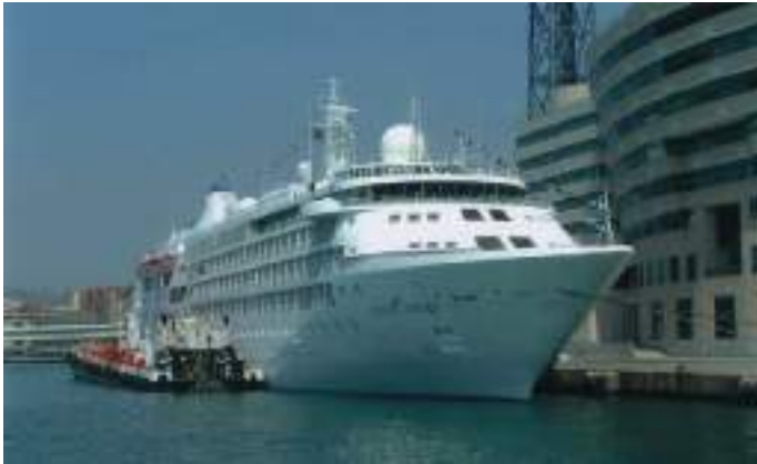
Plate 275 The passenger ship Silver Wind seen taking bunkers from a barge on her starboard side.
