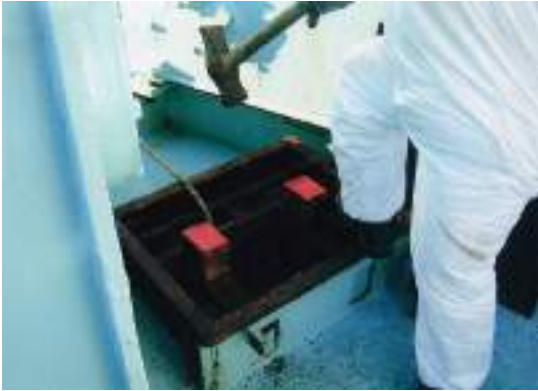
Plate 11 Activating the quick release by a hammer blow to the tapered securing bolt of the bitter end of the anchor cables
