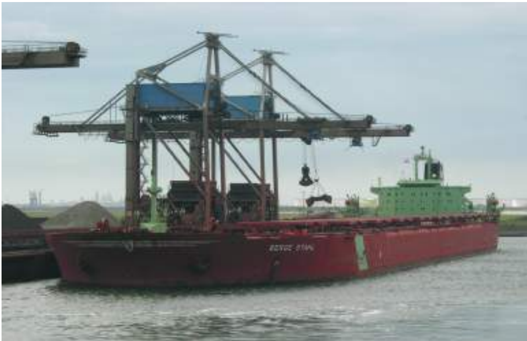
Plate 73 The Berge Stahl bulk carrier, seen alongside in Sept Isles, Canada loading ore by means of bucket grabs from the overhead gantry cranes.
