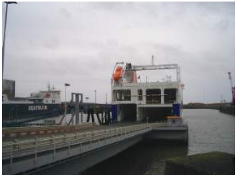
Plate 60 Road ramp and stern opening for a main vehicle deck and a drive-on ramp to an upper exposed vehicle deck of the Stena Performer (IMO 9506227). The vessel carries 151 trailers over three decks and is engaged on the Irish Sea Trade.
