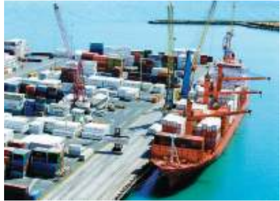
Plate 52 A container vessel lies alongside the container terminal, in Napier New Zealand, loading dock. The ship's own cranes are seen turned outboard so as not to interfere with the shoreside loading cranes.
