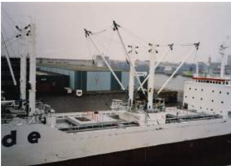
Plate 25 Derricks rigged in union purchase either side of the amidships masthouse. All derricks are employing schooner guys and supported from Samson posts.
