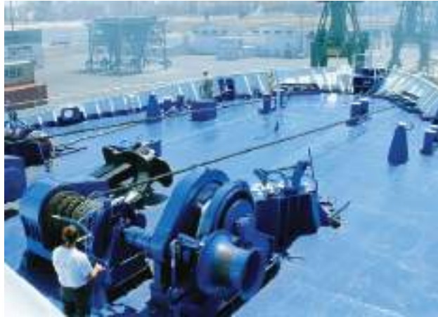
Plate 18 Forward mooring deck of a passenger vessel with separate port/starboard windlass.
