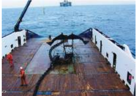
Plate 12 A 15-tonne Stevpris anchor is recovered to the aft deck of an anchor handling vessel in the North Sea offshore operational region.
