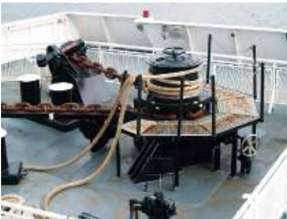
Plate 17 Motorized capstan with gypsy and warping drum, seen at the aft end mooring deck. (Source: Shutterstock.)
