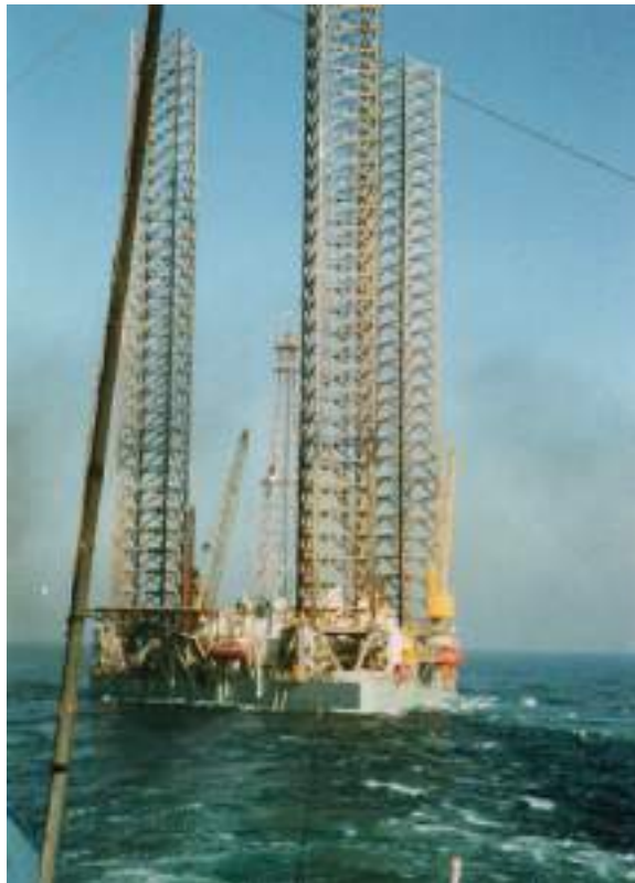
Plate 174 A jack-up mobile drilling rig under tow towards an operational site. Once in position the supporting structure legs are lowered to the sea bed.
