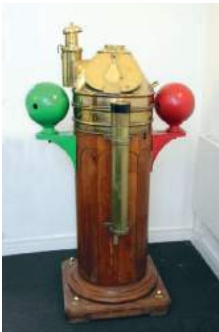
Plate 140 The forward face of a hardwood finish binnacle with ‘helmet’ in place over the compass bowl position.
