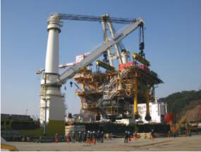
Plate 41 The Happy Star , one of 'Big Lift's' heavy lift vessels, engages in a tandem lift using lifting spreader beams to load an upper deck module for an offshore oil installation.
