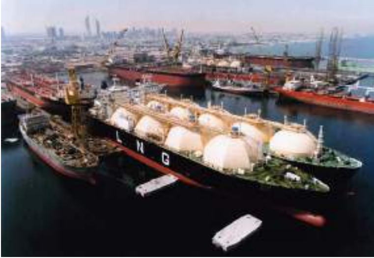
Plate 213 Two LNG carriers lie alongside each other outside the Dubia shipyard. Prominent features are the gas dome structures on the upper decks.
