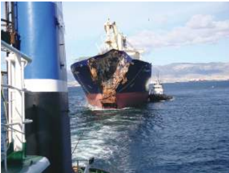
Plate 248 Damaged vessel seen under tow where a chain bridle has been employed.
