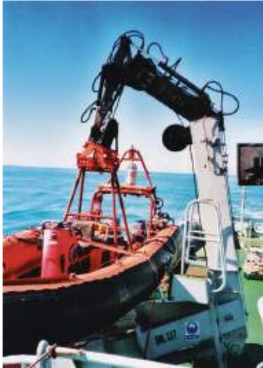
Plate 114 Hydraulic single-arm launching system, for a semi-rigid, fast rescue craft. Operates up to 2.5 tons SWL. The boat is gripped in by quick release web straps and provided with a crew boarding platform.
