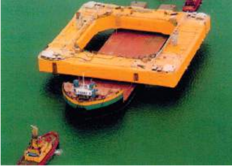
Plate 35 The Giant 4 , cargo barge seen transporting an offshore load with tug escorts in attendance to an offshore platform under construction. Where the loading or discharge is scheduled to take place in tidal waters then respective times and heights of high and low water levels with ebb and flood details would also be required.
