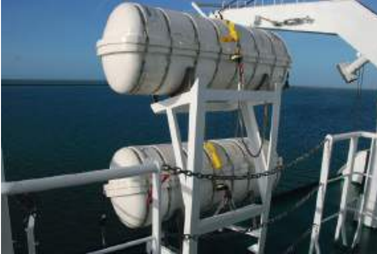
Plate 104 Inflatable life raft stowed in cradle and fitted with disposable hydrostatic release unit.
