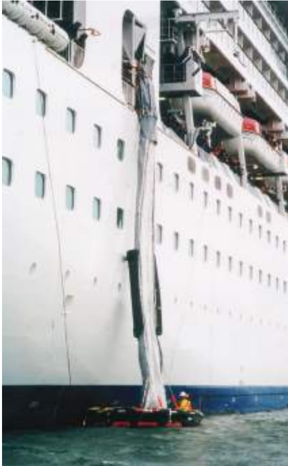
Plate 107 Single chute shown deployed with the surface landing platform.
