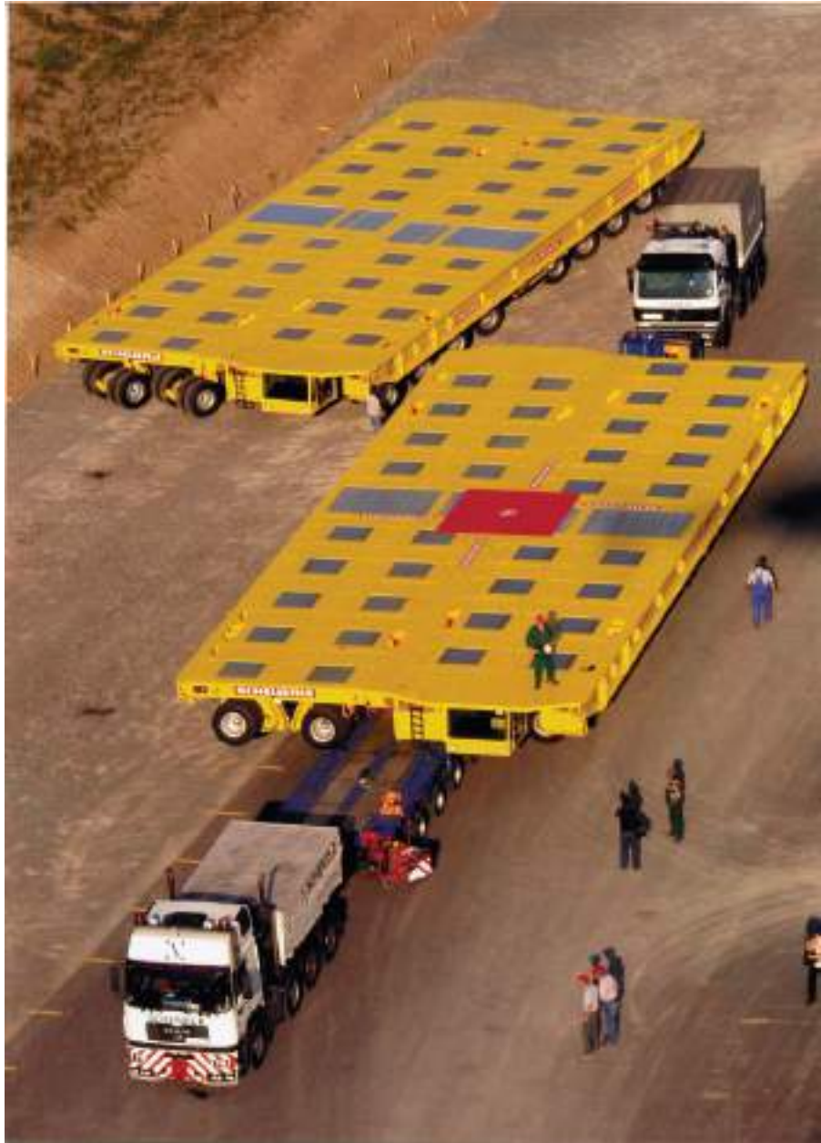
Plate 37 Multi-wheel, self-drive, sectioned road transporter, for shoreside movement of project type cargoes.
