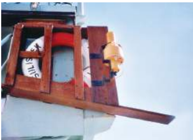
Plate 199 Emergency bridge lifebuoy for use in 'man overboard' emergencies, with combined light and smoke float attached. This one is secured in the stowage bracket on the after side of the starboard bridge wing.
