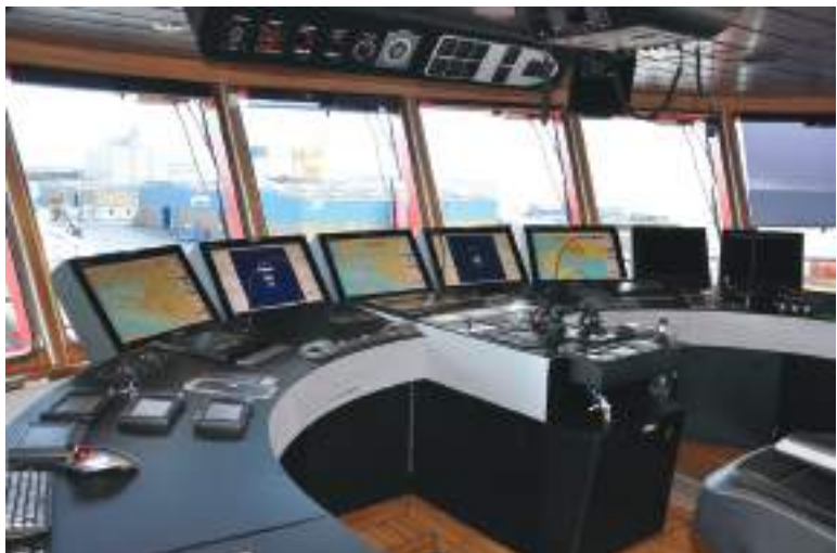
Plate 126 Example bridge layout as seen looking forward through the bridge windows from the autopilot/steering position. Communication console are set either side of centre. (Source: Raytheon Anschutz GmbH.)
