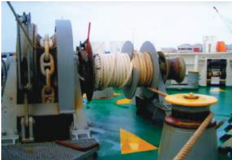
Plate 22 Combined windlass and warping drums rove with a dyneema mooring line.
