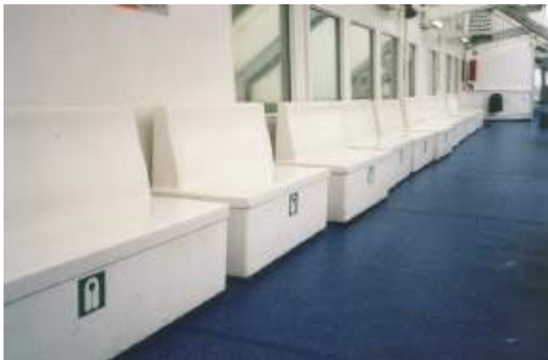
Plate 109 Lifejacket stowage arrangement inside deck seats, on the embarkation deck of a passenger ferry.
