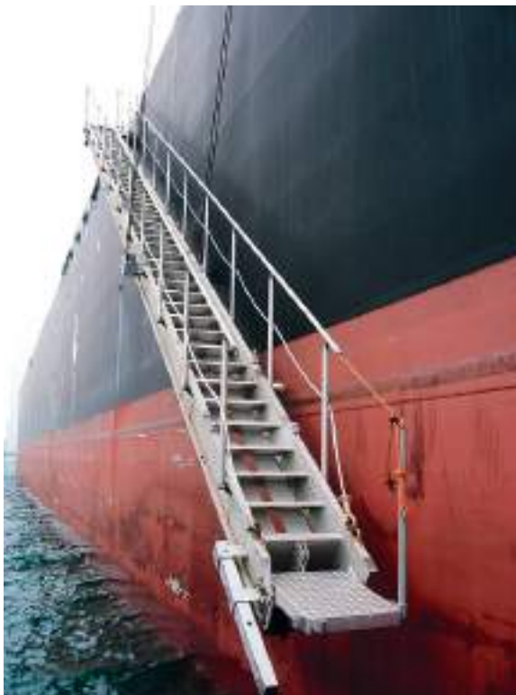
Plate 131 Accommodation ladder seen in the turned out position and deployed with the vessel at anchor. Accommodation ladders should not be rigged more than 55° from the horizontal. (Source: Shutterstock.)
