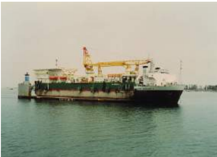
Plate 34a The heavy lift vessel Super Servant 3 engages in project cargo operations by transporting the offshore barge Al-Baraka 1 .
