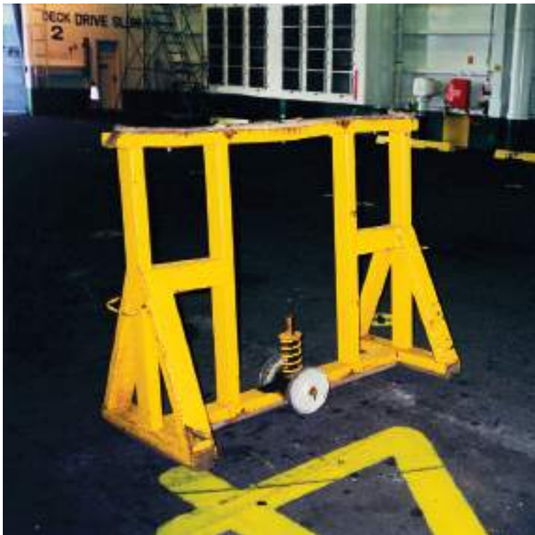
Plate 62 Example of trestle support, for landing ro-ro drop-units.
