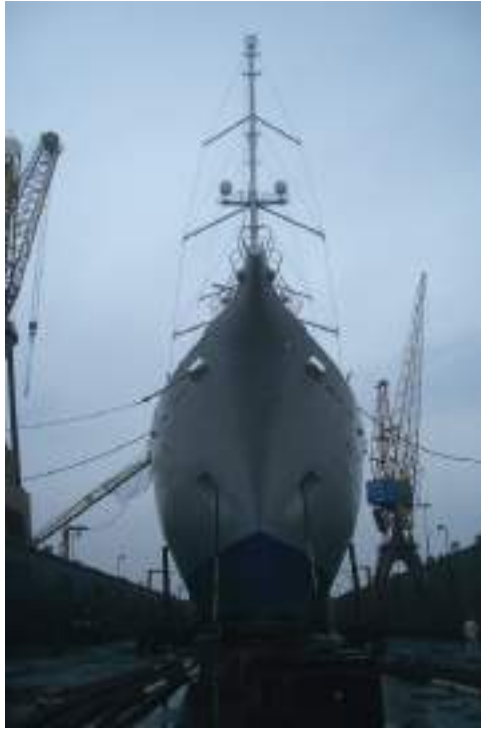
Plate 191 The cleaned and coated hull of the Wind Surf seen in the dry dock complex at Lisnave, Portugal.
