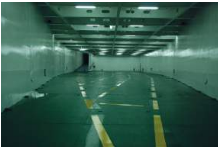
Plate 215 Example 'Lower hold' vehicle deck, seen with allocated metres lanes for maximum vehicle stowage. Lower holds may provide access by descending ramp from a main deck position or by means of a mechanical electro/hydraulic central lift.
