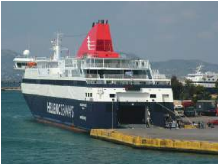
Plate 59 Stern door arrangement of Nissos Mykonos vehicle ferry, seen stern to a ro-ro berth.
