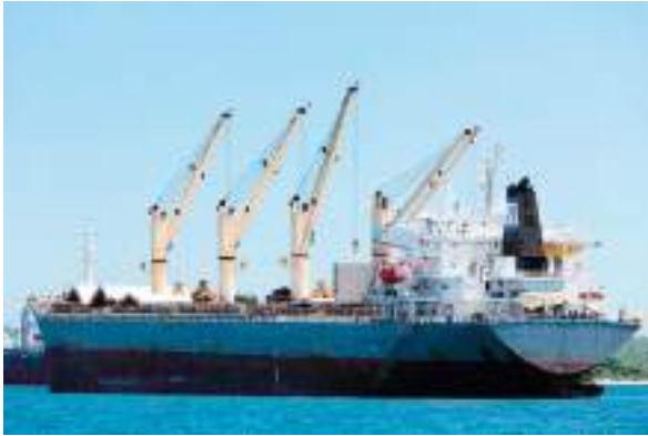
Plate 51 Dry cargo vessel with prominent deck cranes deployed. (Source: Shutterstock.)
