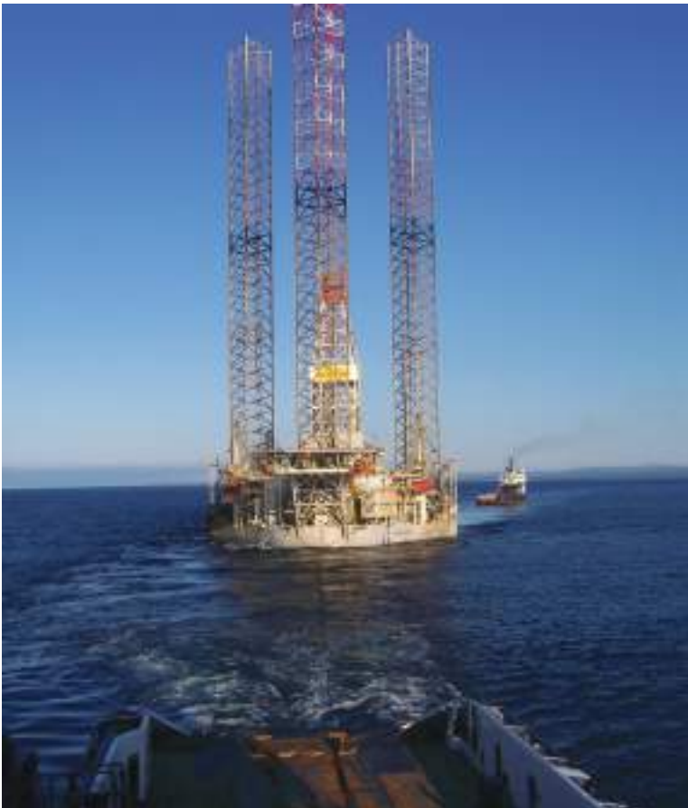
Plate 252 The jack-up rig Santa Fee-Magellan , seen under tow by means of a wire bridle, from the Cromarty Forth, as seen from the deck of brake tug.
