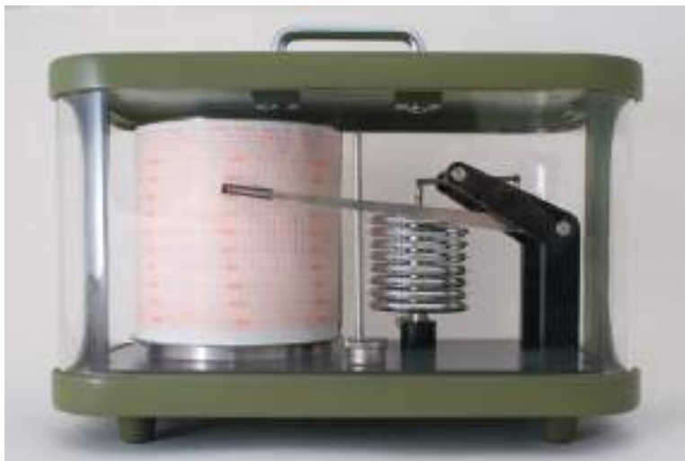
Plate 152 Marine barograph. This instrument provides a graphical presentation of 'barometric tendency'. (Source: Shutterstock.)
