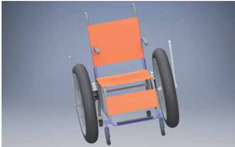
Figure 14. Final wide wheel design.
