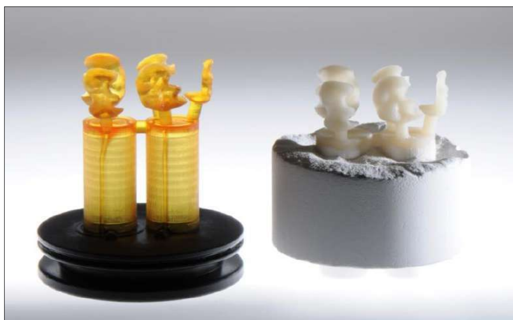
Figure 17. Comparison of 3D printed and pressed ceramic inlays.
