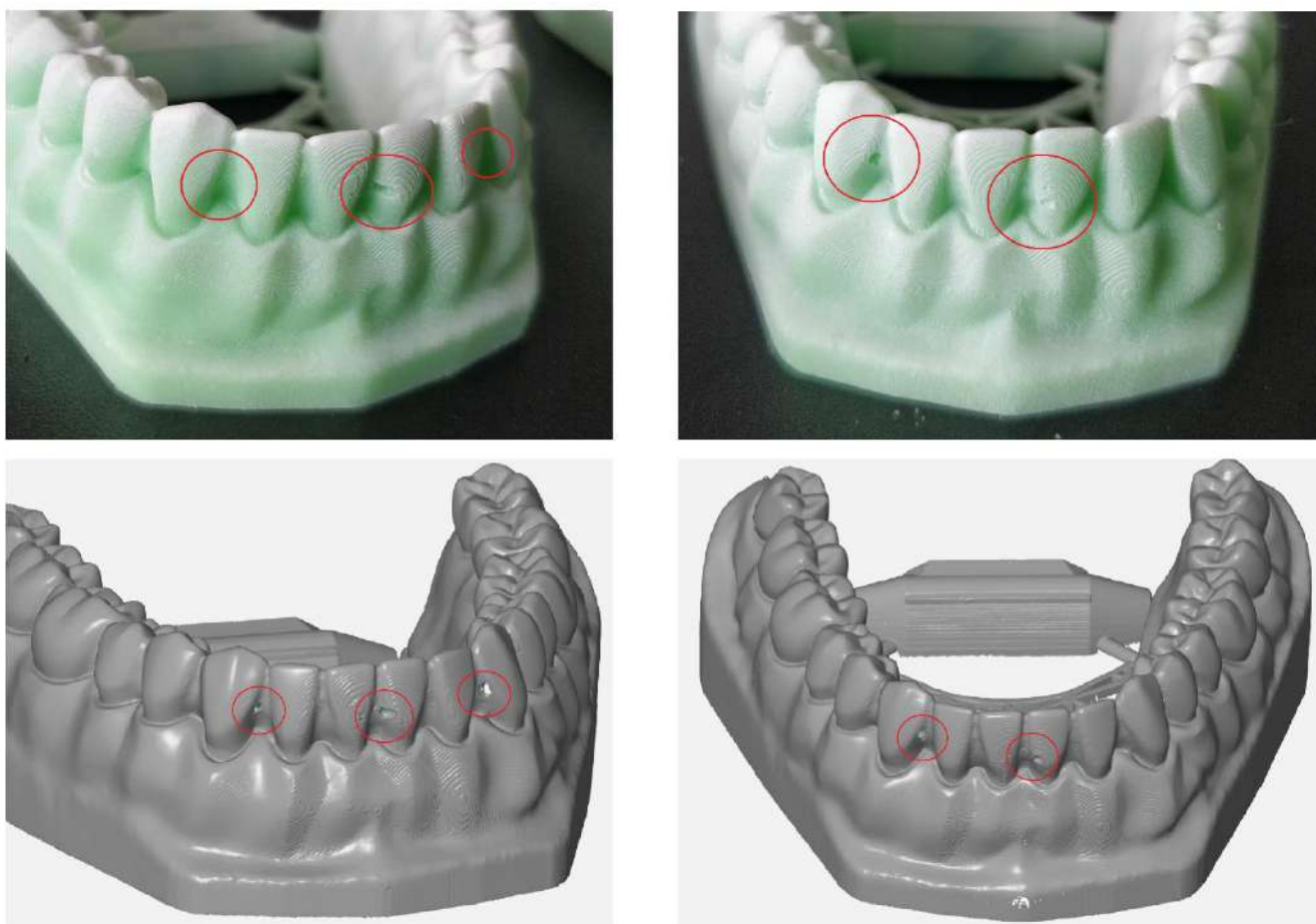
Figure 7. Defects, shown in red circles, in two models printed with the material from Producer 3 visible in the resulting scan.
