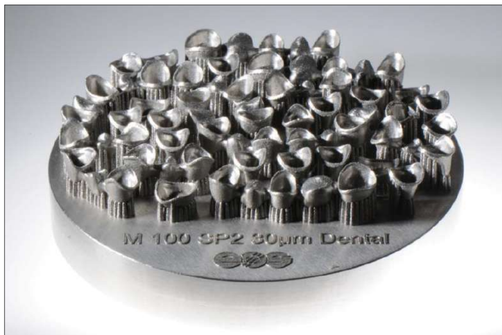
Figure 3. Lasersintered CoCr Crowns and Bridges.
