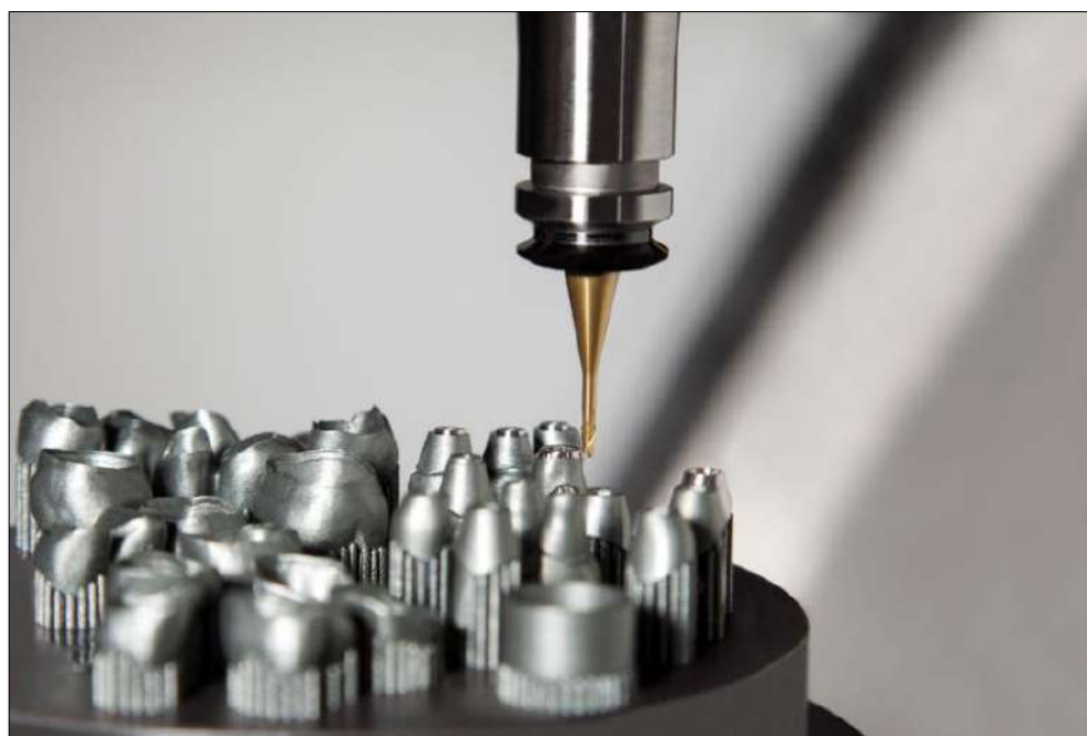
Figure 5. Hybrid manufacturing combines additive manufacturing. With CNC-milling (Source: Datron AG, Mühlthal, Germany).
