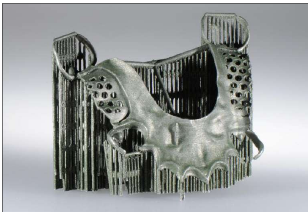
Figure 4. Laser sintered removable partial denture with support structures.
