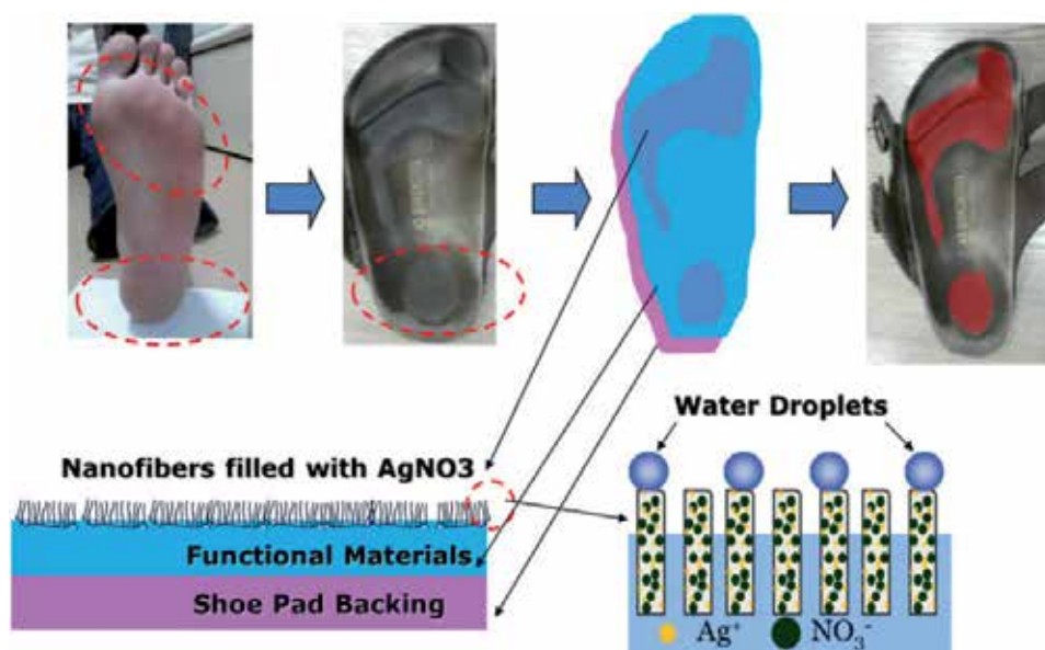
Fig. 17. Proposed Structure of an Eco-Product Required Biocides for a Shoe Pad (Adopted from Lem et al., 2011)
