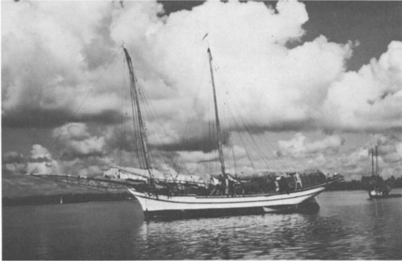
Plate 5. The perahu pinas gobel is distinguished by its cruiser stern and clipper bow, perhaps copied from an eighteenth century French pinasse .
