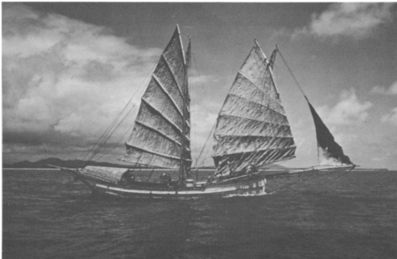
Plate 6. The perahu pinas dogor under sail makes use of dipping lug sails, made of mengkuang reed matting, stiffened with battens.
