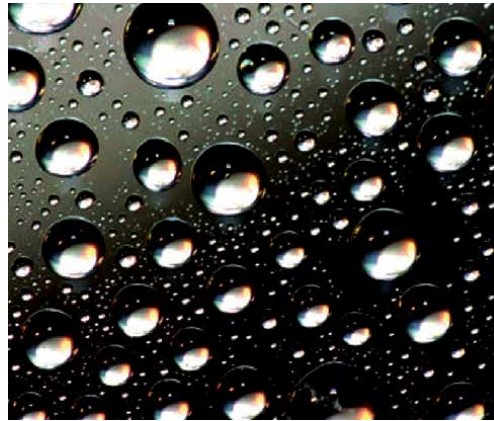
Figure 10. Self-cleaning and anti-reflective nanocoatings [7].
