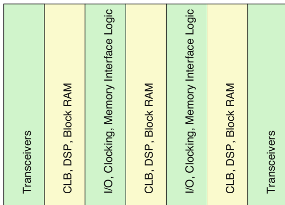
Fig. 3.38 Floor-plan of column-based Xilinx® UltraScale FPGAs
