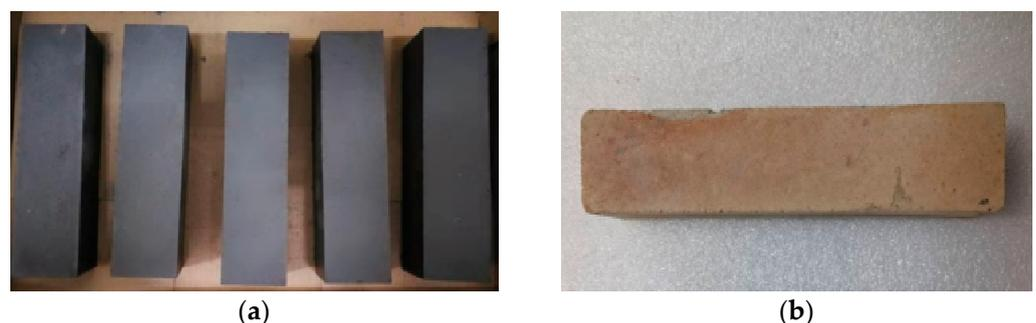
Figure 4. Bricks before and after sintering: (a) Unsintered bricks, (b) Sintered brick.
