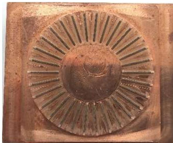
**Figure 1.** Electrode for preparing texture.
