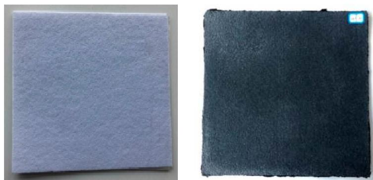
**Figure 3.** Physical images: (a) PET needle punched nonwoven fabric; (b) Microwave-absorbing impregnated nonwoven fabric.
