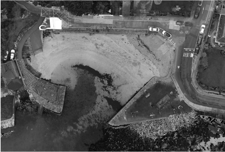
Figure 5.1 Photomosaic plan of Sandy Cove Harbour, Dublin, assembled from drone images. Image reproduced with permission from Geomap.
