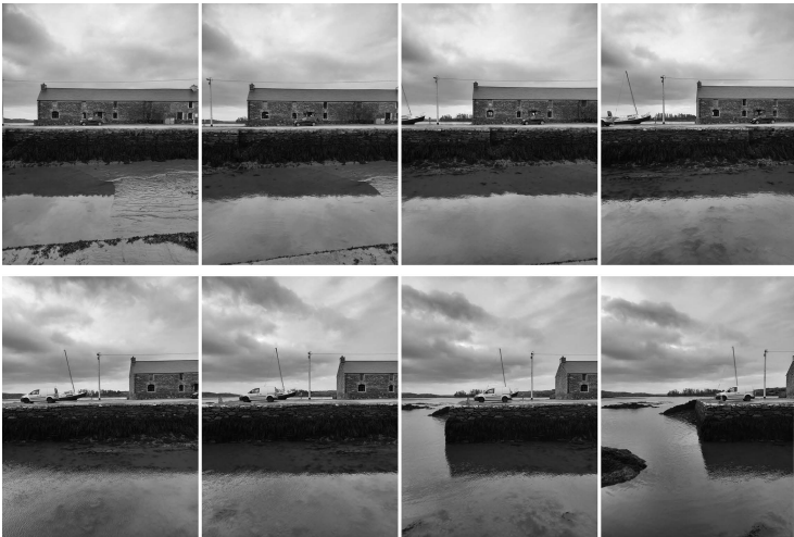
Figure 7.4 A series of rectified photos taken by Sarah Canty, helped by Anke Eckardt, used to produce an elevation of the Quay and buildings in 2021.
