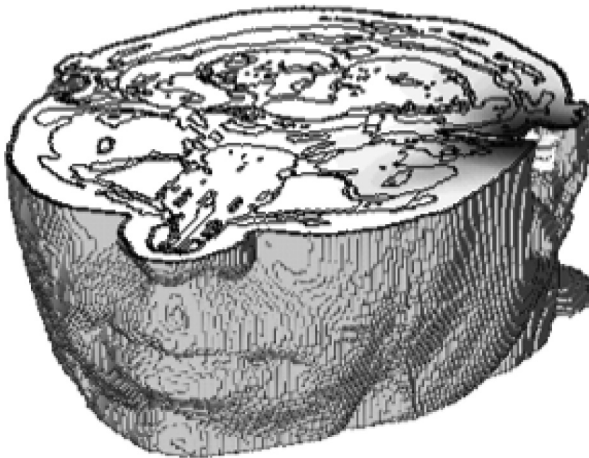
FIGURE 6.8 Intracorporal SAR distribution in a cross-section through an in-the-ear hearing aid, caused by the telecommunication link to a belt-worn transmitter. Voxel SAR values are in the nanowatt per kilogram range.
