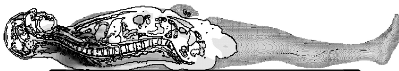
FIGURE 6.3 Intracorporal current density distribution induced by a patient heating blanket. (Data from Leitgeb, N. 2010. Safety of Electromedical Devices. Law-Risks-Opportunities . Vienna, Austria: Springer. With permission.)
