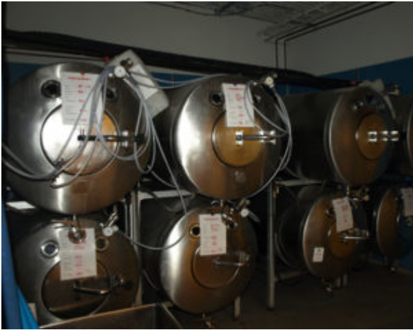
Figure 7 Fermentation of grape juice to make wine produces CO 2 as a byproduct. Fermentation tanks have valves so that pressure inside the tanks can be released.
