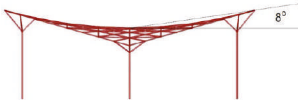
Figure 6. Determination of the roof inclination angle.
