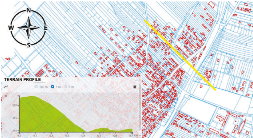
Figure 2. Cross-section through the northern section of Radzionków's urban zone—the difference in elevation between the central and valley part is around 32 m; the terrain has a northwest-facing slope with an incline of around 7%. (Original work based on data from https://mapy.geoportal.gov.pl ).
