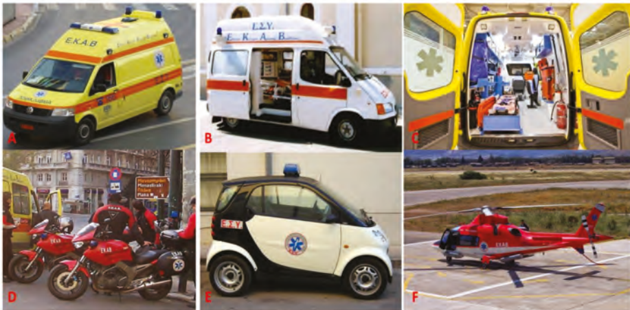
Figure 2. Types of EKAB ambulances. (A,B) Basic type of Ambulance; (C) Mobile Intensive Care Units; (D) Motorcycle ambulances; (E) Small vehicles for minor roads; (F) Helicopters.
