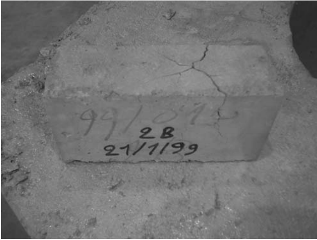
Figure 3.2 Disintegration of a concrete block containing non-stabilized slag particles.
