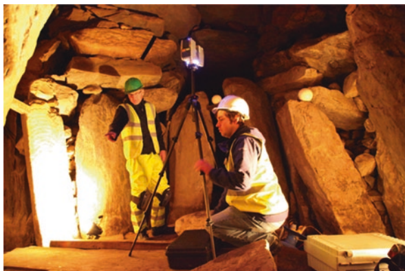
Fig. 10.1 Recording the 3D structure of one the internal tombs at Knowth, BrúnaBóinne using a terrestrial laser scanner. (© The Discovery Programme)
