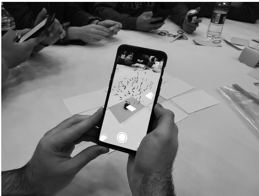
Figure 14.5 An undergraduate physics student plots the field around a small stack of magnets.
