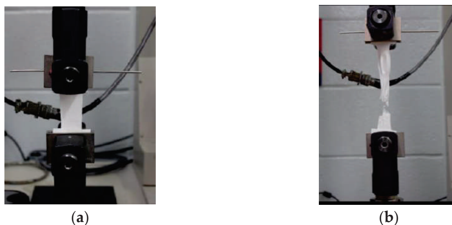
Figure 6. Electrospun membrane specimen (a) loaded onto the Sintech 2/G materials testing system for uniaxial tensile testing, and (b) tested till failure.
