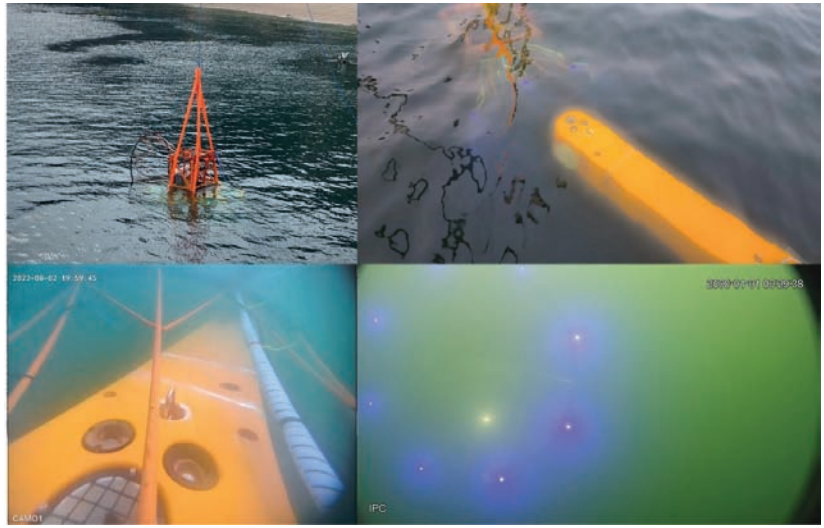
Figure 14. Autonomous docking tests in the shallow sea.
