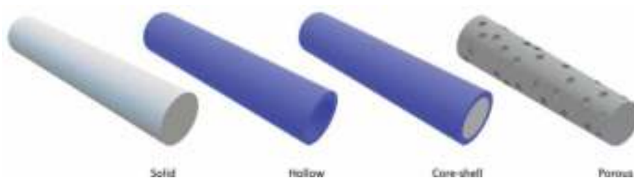
Figure 5. Possible morphologies of nanofibers obtained by electrospinning.
