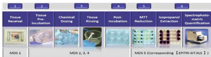
Fig. 1. Protocol of skin irritation test (SIT) developed by ITRI for EPiTRI ®
