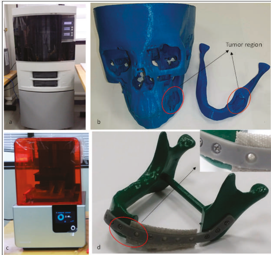
Figure 8. (a) Fused Deposition Modeling machine with its fabricated polymer model (b) indicating the tumor region and (c) SLA machine and its produced mandibular scaffold (d) with a close-up view.
