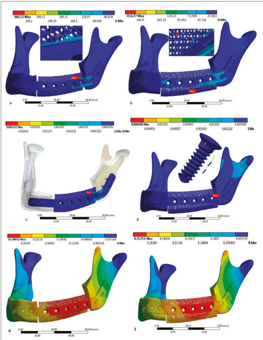
Figure 14. Von Mises stress (top), strain (middle) and deformation (bottom) distribution of mandibular framework model with two scaffolds (a,c,e) inner porous and (b,d,f) top and bottom porous plate.
