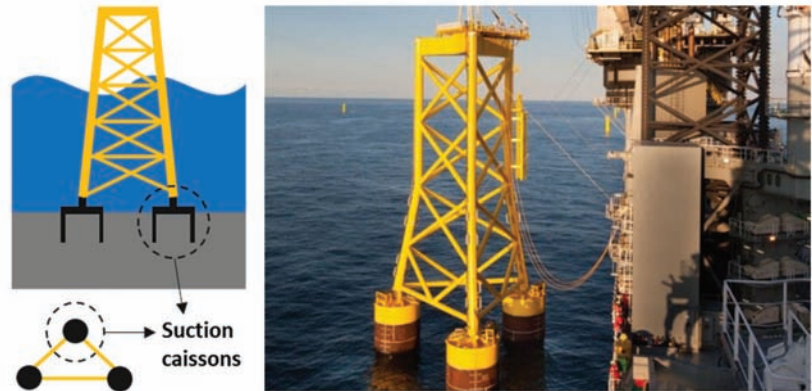
Figure 1. Schematic of a 3-legged jacket on suction caissons reproduced from [6], with permission from Ørsted, 2019.
