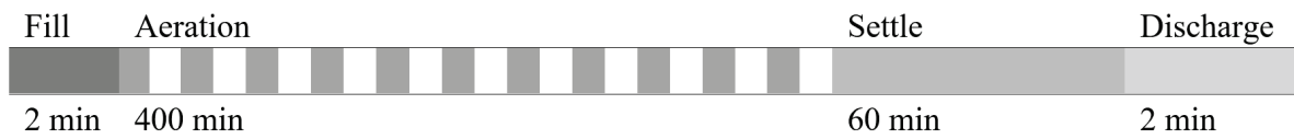
Figure 3. Illustration of cycle sequence (the on-off aeration pattern is demonstrated using the grey and white sequence in the aeration period).
