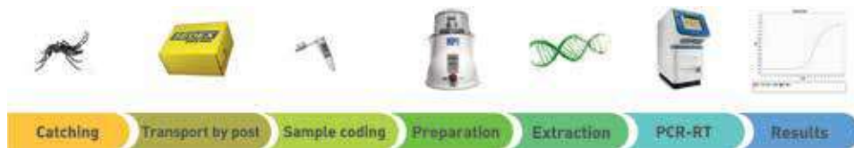
Figure 8. Logistic of the Integrated Monitoring Virus (MI-Virus). Weekly, caught female Aedes aegypti by MosquiTRAP are placed in barcoded Eppendorf tube and send by post to laboratory for RT-PCR analysis. Bar code provides GIS trap position. Source: Ecovec Company, Belo Horizonte, Minas Gerais State, Brazil.
