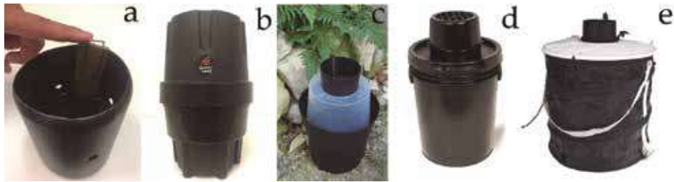
Figure 2. Passive mosquito traps used for surveillance: (a) ovitrap, (b) MosquiTRAP, (c) Aedes Gravid Traps (GAT) , (d) Autocidal Gravid Ovitrap (CDC-AGO) , and (e) the active trap BG-Sentinel .
