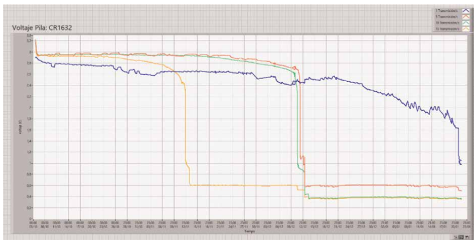
Figure 18. Battery discharge voltage curve versus time and number of transmissions/s; blue: 1 transmission/s, red: 5 transmissions/s, green: 10 transmissions/s, and yellow: 15 transmissions/s.
