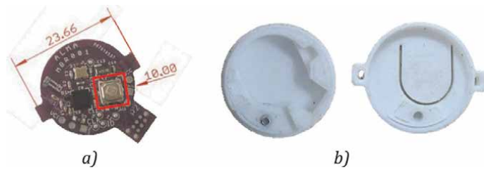
Figure 6. Photograph of the designed prototype and case: a) electronic device and b) thermoplastic structure made using a 3D printer.
