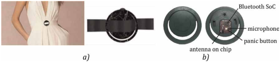
Figure 9. Device hidden in a belt: a) design of the accessory and b) prototype made of plastic with the electronic device inserted.
