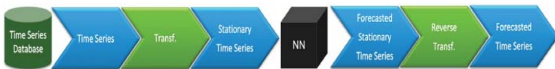
Fig. 2. The process of non-stationary time series forecasting.
