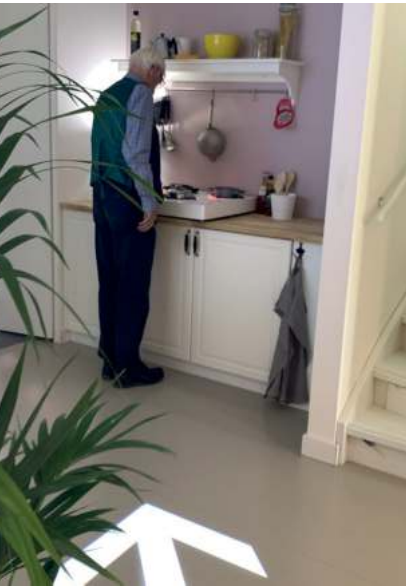
Figure 3 (left) Dinner time. The arrow on the floor lights up, and the directions in the kitchen help the inhabitant prepare the food.
