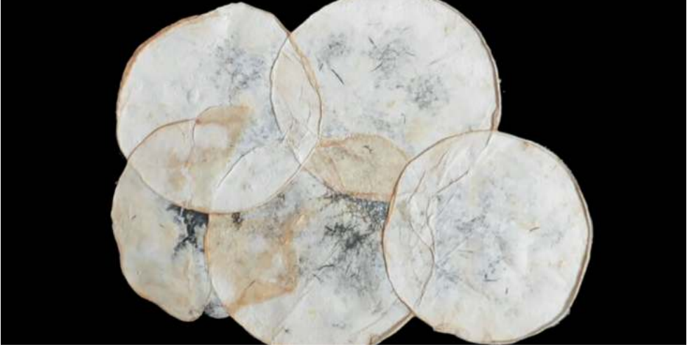
Figure 1 NEFFA (Aniela Hoitink), MycTeX©, a seamless production method that helps create custom-made clothing from compostable mycelium (photo: NEFFA).
