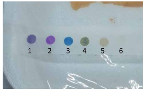
Figure 4. An example of the array placed over the tray containing the poultry meat, with sensors from one to six based on m -cresol purple (1), o -cresol red (2), bromothymol blue (3), thymol blue (4), chlorophenol red (5), and the Ellman's reagent (6).
