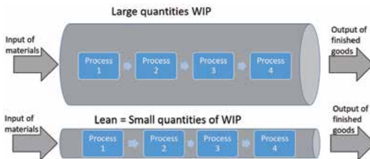
Figure 2. The physical “leanness” observed with low levels of WIP.
