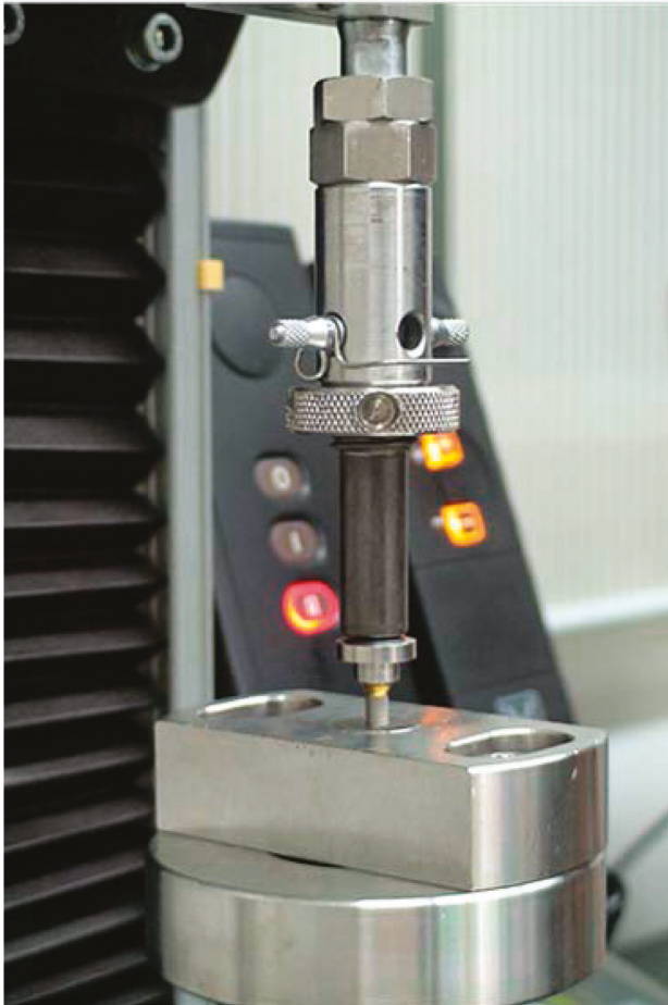
Figure 3. Loading machine and customized jig (Instron 8841, Instron Corp., Mass, Norwood MA, USA).
