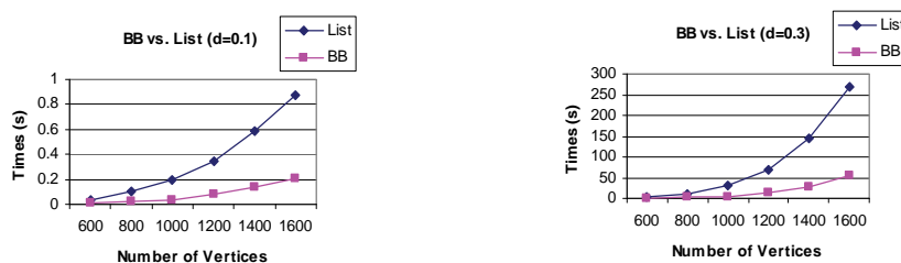
Figure 6. Time results for a bit-parallel (BB) and a classical (list) implementation of a naïve MCP algorithm with a classical vertex coloring strategy to establish bounds.
