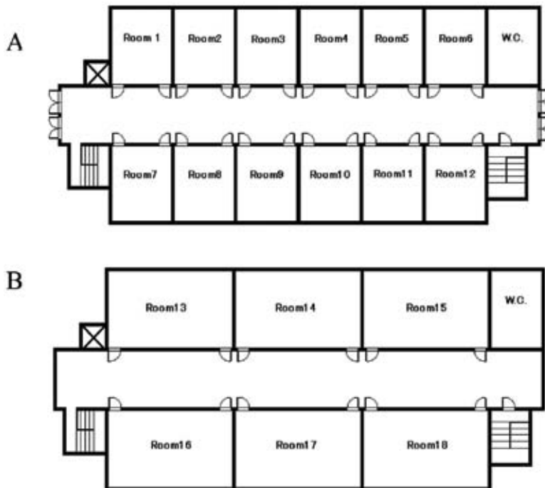
Fig. 6. Layout of the simulated public facility: A - 1 st floor, B - 2 nd and 3 rd floors
