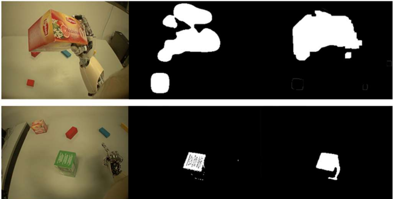
FIGURE 14 | Segmentation improvements for two objects after interaction. On the left, the robot's view of the scene. The middle column shows the first segmentation generated from the "static scene baseline." The last column shows the improved segmentation after learning continued with new images collected during the manipulation of the object.
