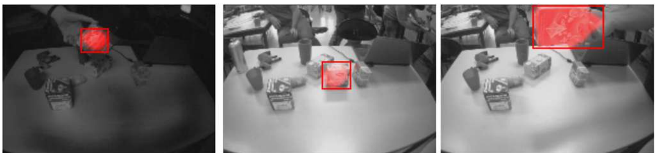
FIGURE 1 | During a stereotypical manipulation task, object detection is a hard but critical problem to solve. These images collected during our experiments show the changes in lighting, occlusions, and pose of complex objects. (Note: best viewed in color) We provide a framework that allows for the easy integration of multiple, new detectors (Leitner et al., 2013a).
